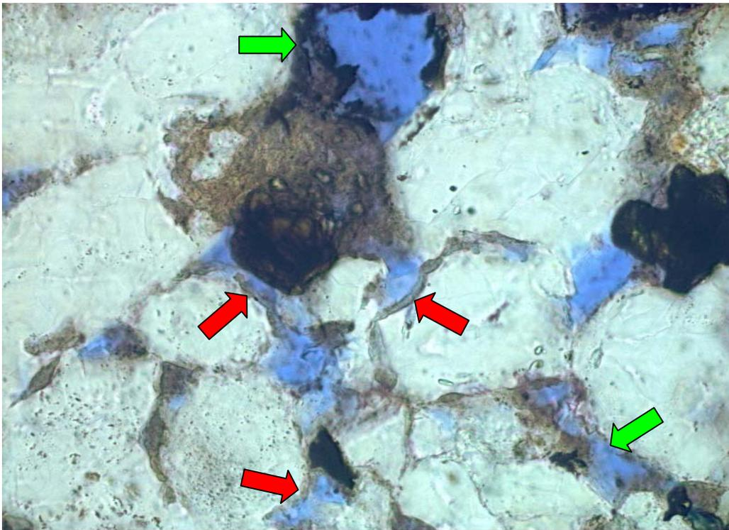
H-23 5408.5m Chlor rims; leached clasts; chlor clast; TiO<sub>2</sub>; intergr pores — 0.010 mm
