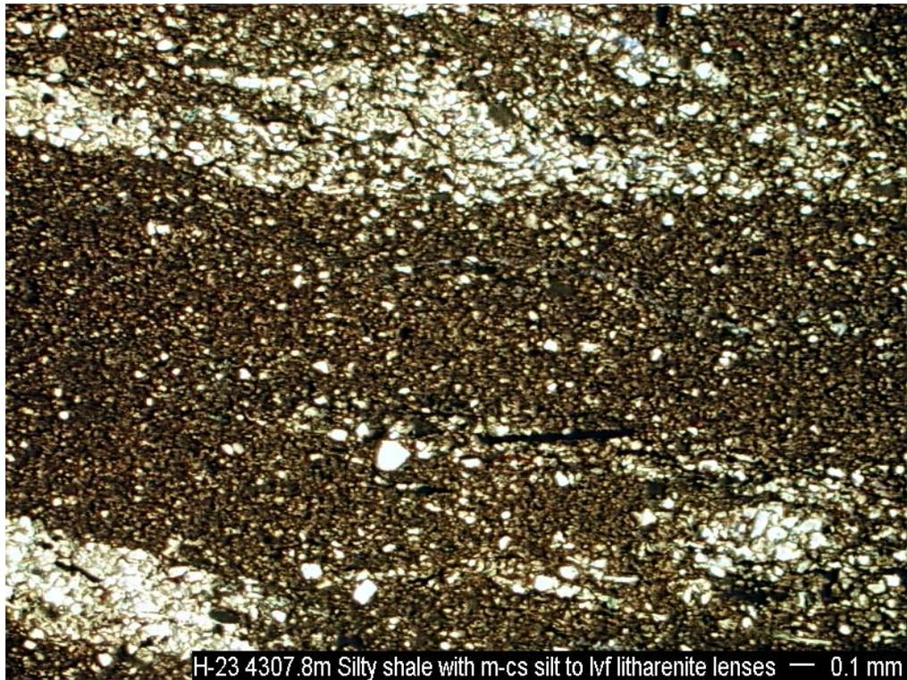
H-23 4307.8m Silty shale with m-cs silt to lvf litharenite lenses — 0.1 mm
