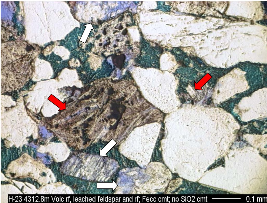
**5 and 6)** Same field of view under plane polarized light (5) and under crossed polars (6). Little or no silica cement precipitated before precipitation of pore-filling ferroan calcite. Volcanic rock fragments are common (red arrows). Intragranular porosity and microporosity has formed by partial dissolution of feldspars and rock fragments (white arrows). Unleached microcline (tartan twinning, upper right, photo 6)
