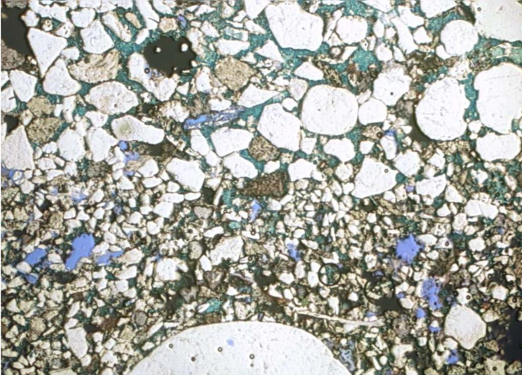
H-23 4312.8m Mw sorted, ang, lvf-lf lith; mod sorted lf-cs lith; Fecc cmted — 0.1 mm
