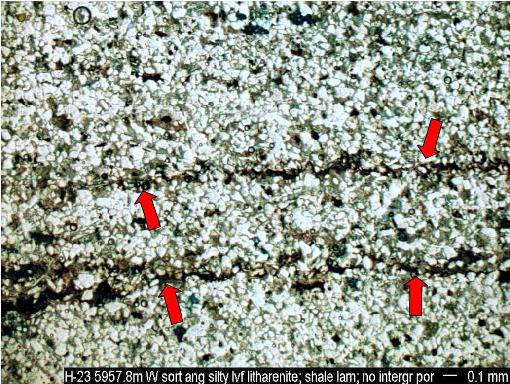
1) and 2) Well sorted, angular silty lower very fine grained litharenite. Well laminated, with local argillaceous/ carbonaceous laminae (red arrows). Intergranular porosity is completely occluded by close grain packing, compaction of ductile clasts and matrix into pores, sutured grain contacts, silica cement and interstitial authigenic chlorite. Labile clasts and detrital matrix clays are often chloritized.
