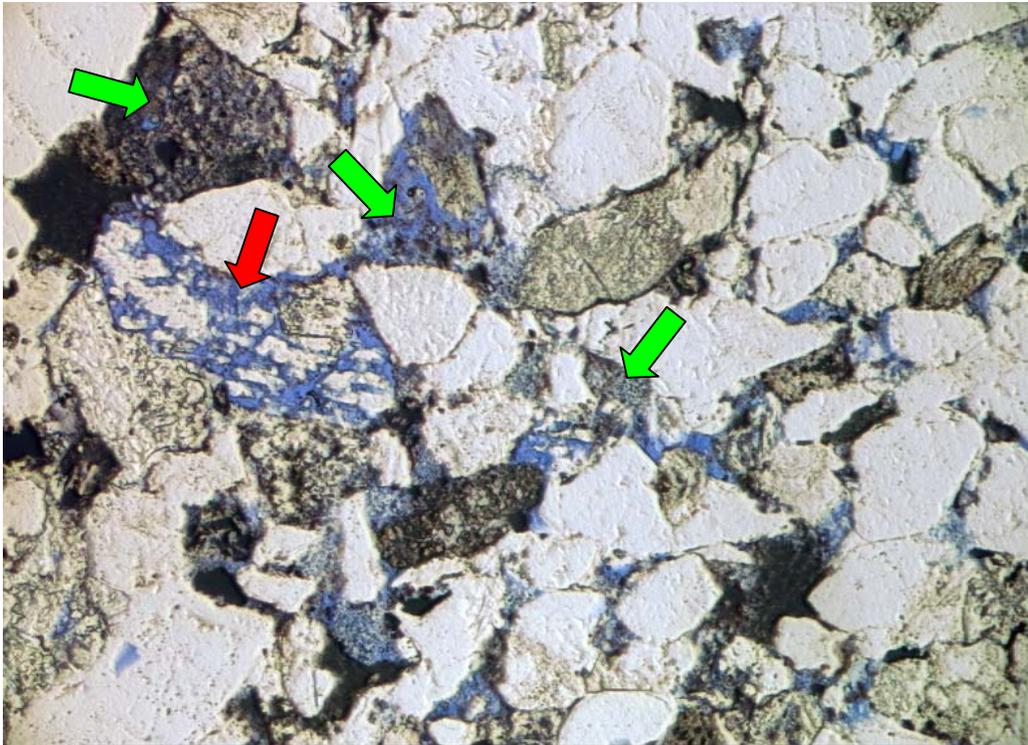
H-23 4349.7m Most porosity is 2ary; micropor in kaol, and lched clasts ——— 0.1 mm
