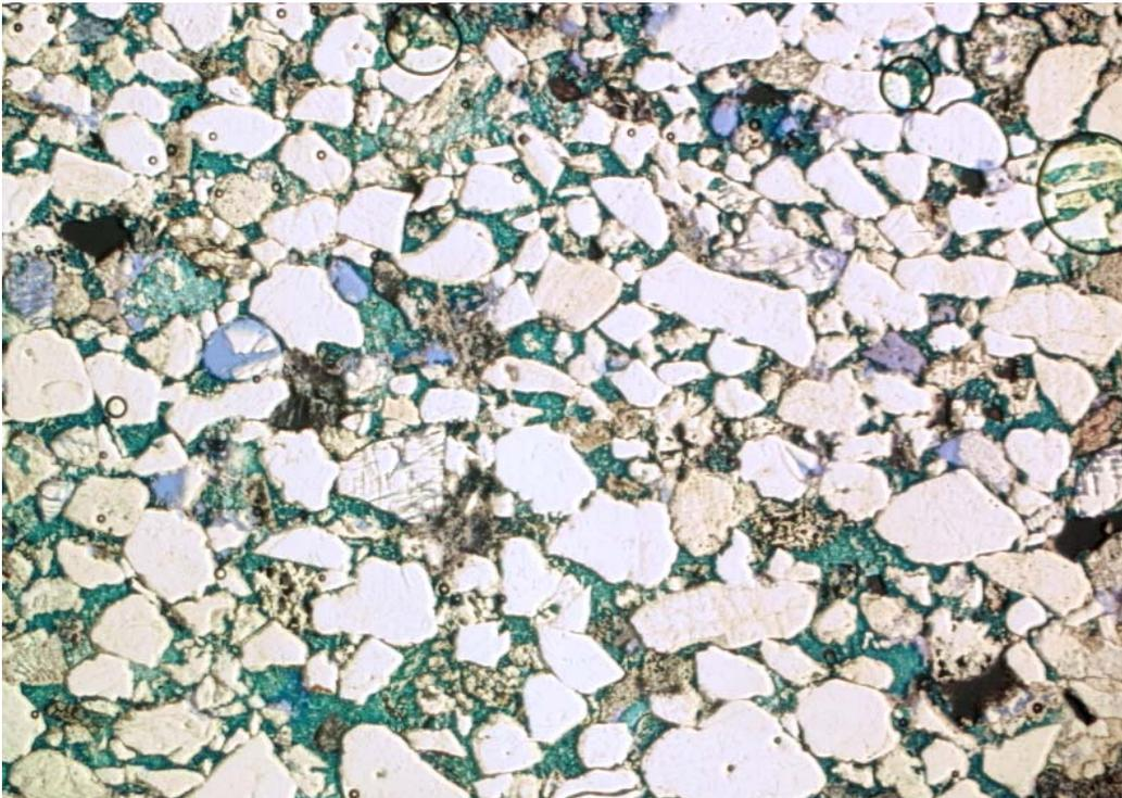
H-23 4312.8m Mod sorted ang-rd vf-lcs Fecc cmted feldspathic lith — 0.1 mm
