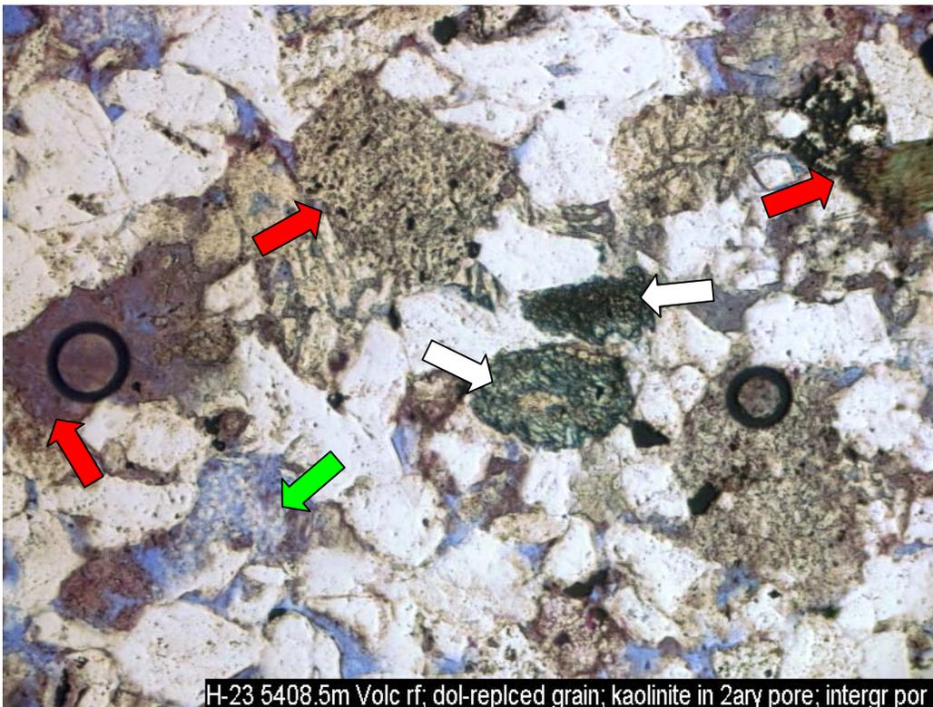
H-23 5408.5m Volc rf; dol-replcd grain; kaolinite in 2ary pore; intergr por
