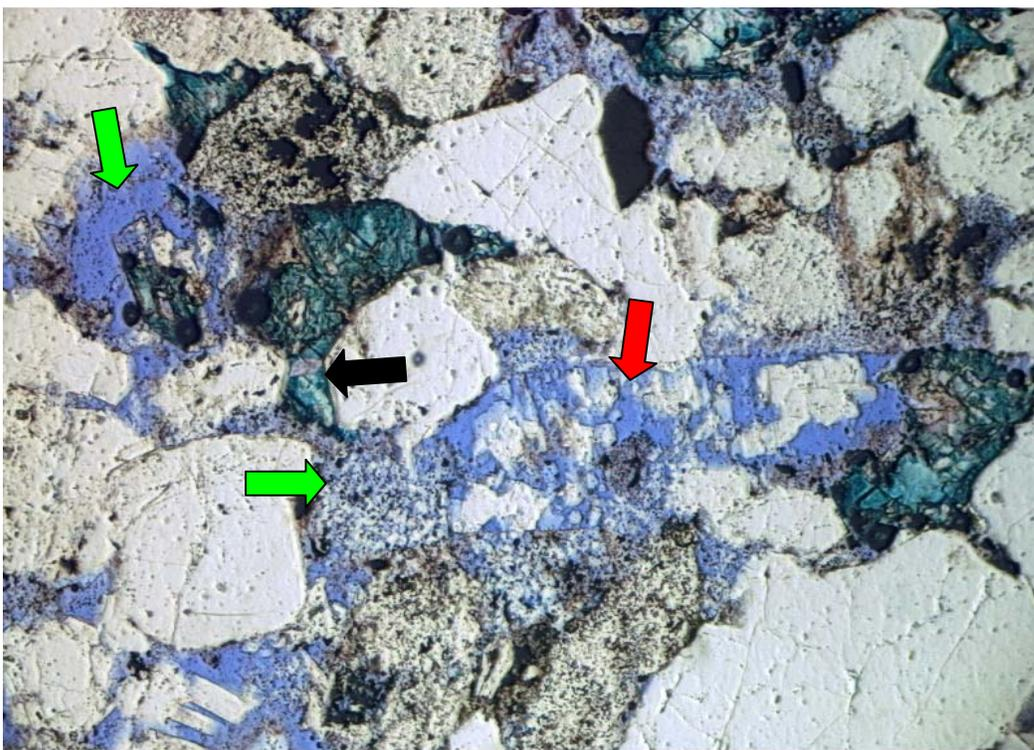
H-23 4354.5m Leached fds and rf; Fecc later than SiO<sub>2</sub> cmt, kaolinite ——— 0.1 mm
