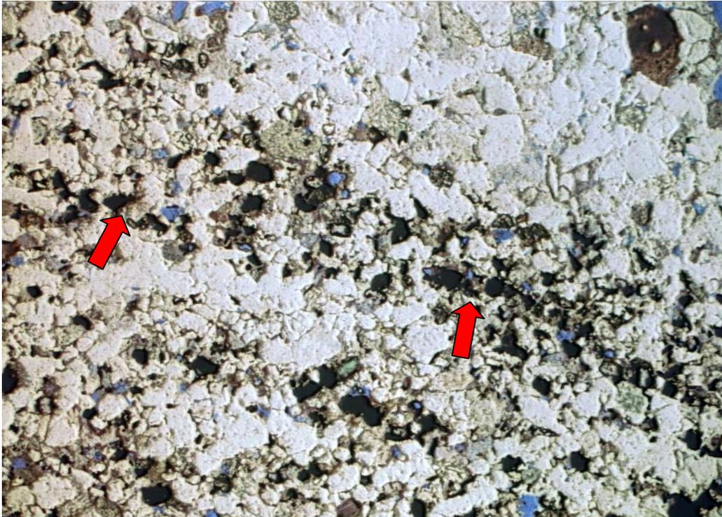
H-23 5406.5m Conc of heavy minerals; SiO<sub>2</sub> cmt: close packing; 0.1 mm
