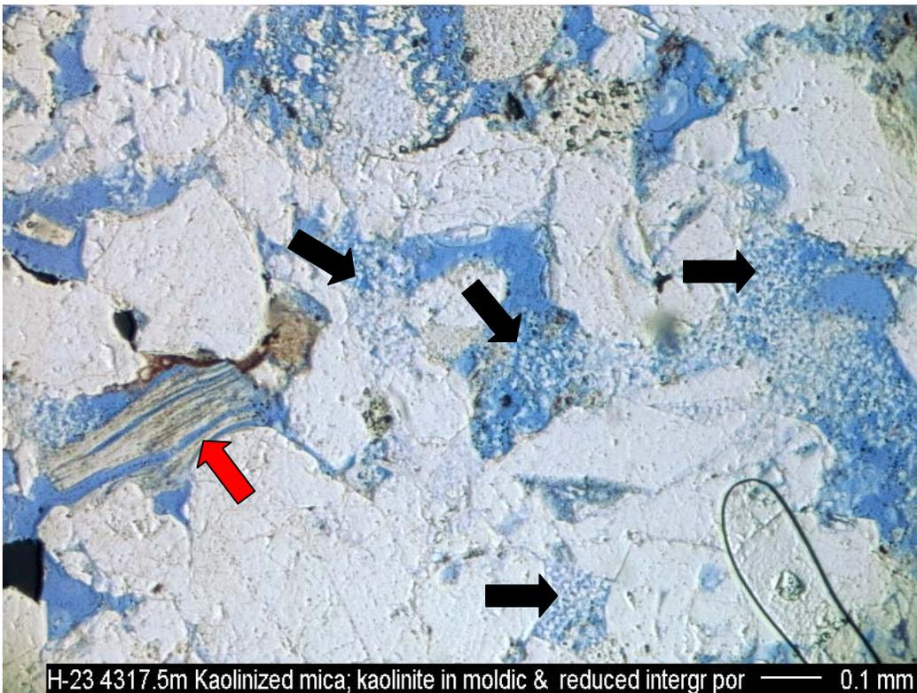
H-23 4317.5m Kaolinized mica; kaolinite in moldic & reduced intergr por ——— 0.1 mm
