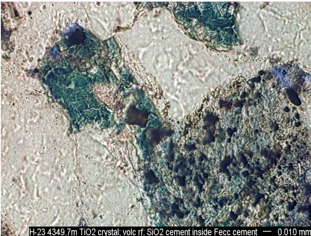
H-23 4349.7m TiO<sub>2</sub> crystal; volc rf; SiO<sub>2</sub> cement inside Fecc cement — 0.010 mm
