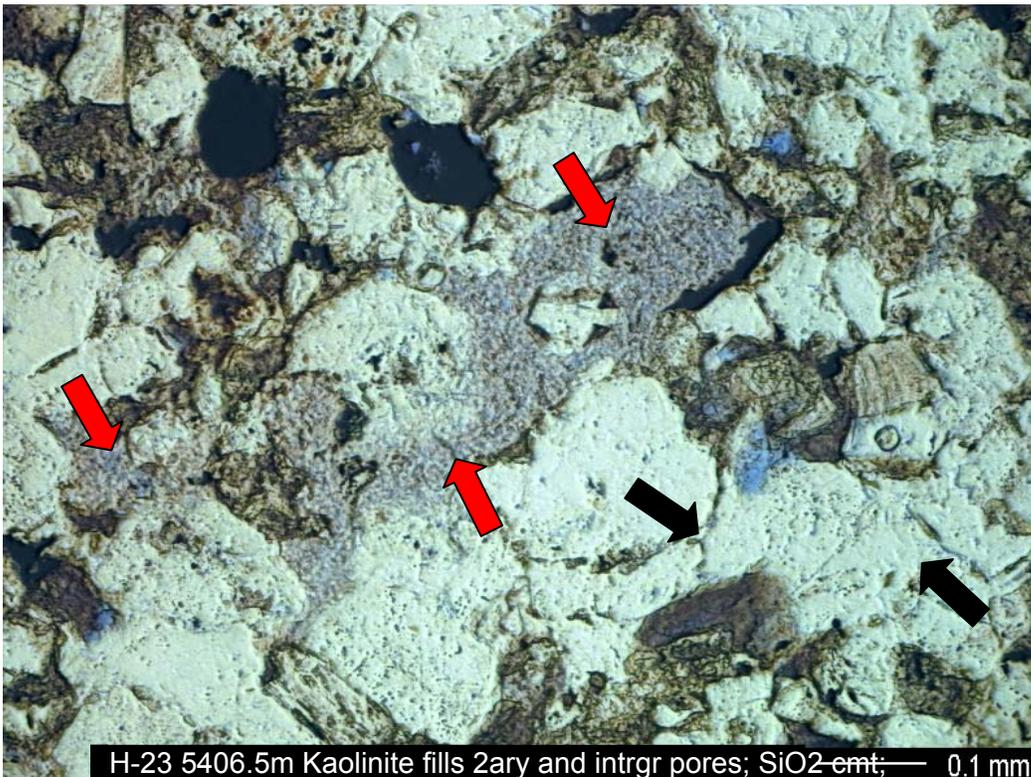
H-23 5406.5m Kaolinite fills 2ary and intrgr pores; SiO<sub>2</sub>-cmt; — 0.1 mm
