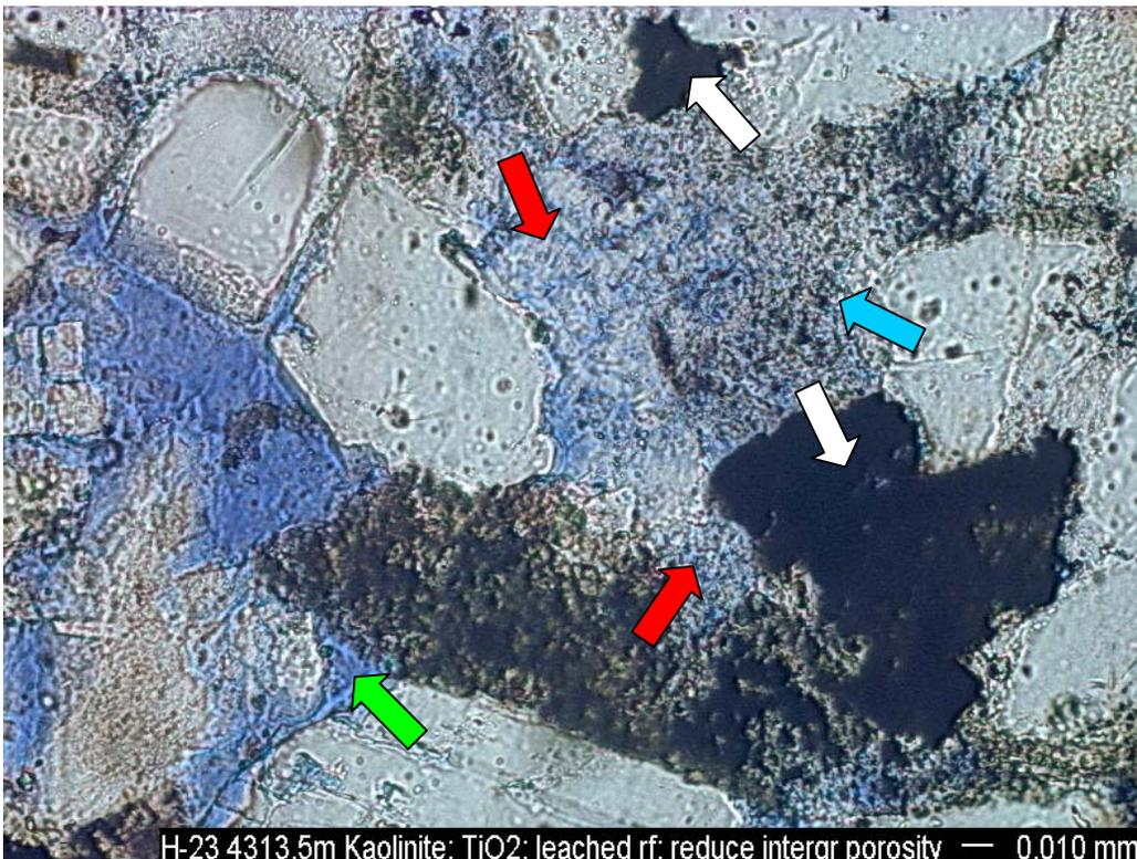
H-23 4313.5m Kaolinite;  $\text{TiO}_2$ ; leached rf; reduce intergr porosity — 0.010 mm
