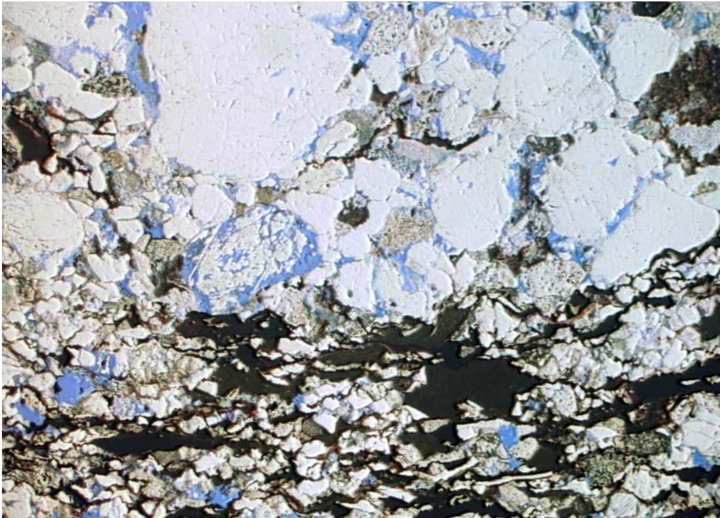
H-23 4318.5m Carbonaceous vf lith overlain by p-m sort lf-lvcs qtzose lith — 0.1 mm
