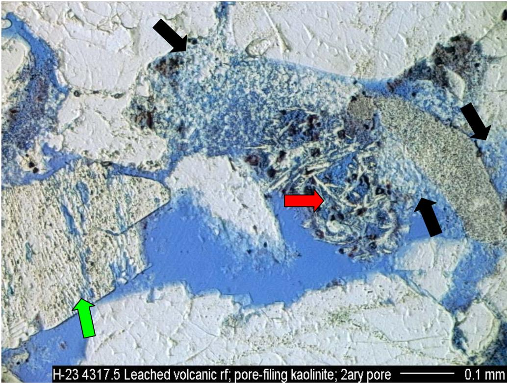
H-23 4317.5 Leached volcanic rf; pore-filling kaolinite; 2ary pore ——— 0.1 mm
