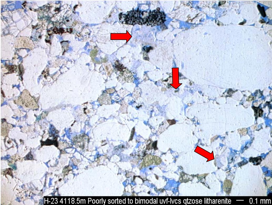
5) and 6) Same field of view under plane polarized light (5) and under crossed polars (6). Poorly sorted to bimodal upper very fine to lower very coarse grained quartzose litharenite. Permeability is reduced by the small average grain size of the more abundant fine grain size fraction, and by abundant pore-filling kaolinite (arrows).
