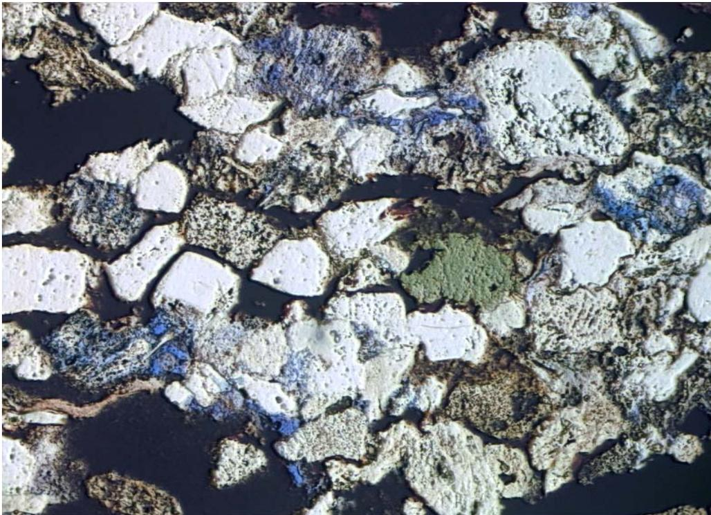
H-23 4313.5m Compacted carb debris, sid clasts; glauc; leached rf, fds ——— 0.1 mm
