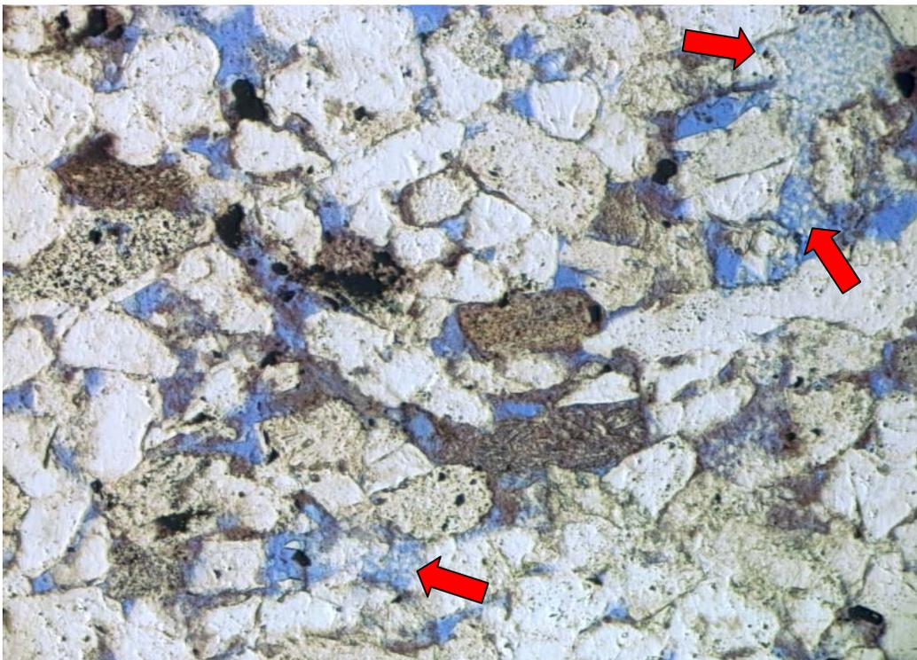
H-23 5407.5m Leached clasts; chlorite rims; kaolinite; good connectivity — 0.1 mm
