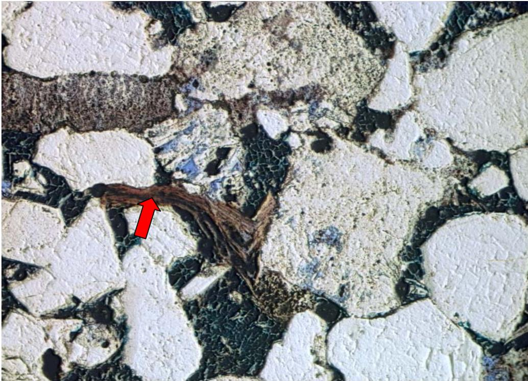
H-23 4319.8m Altered and deformed biotite; leached fds; Fecc cmt ——— 0.1 mm
