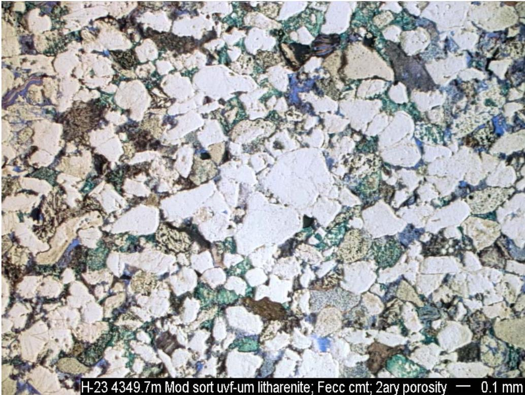
H-23 4349.7m Mod sort uvf-um litharenite; Fecc cmt; 2ary porosity — 0.1 mm
