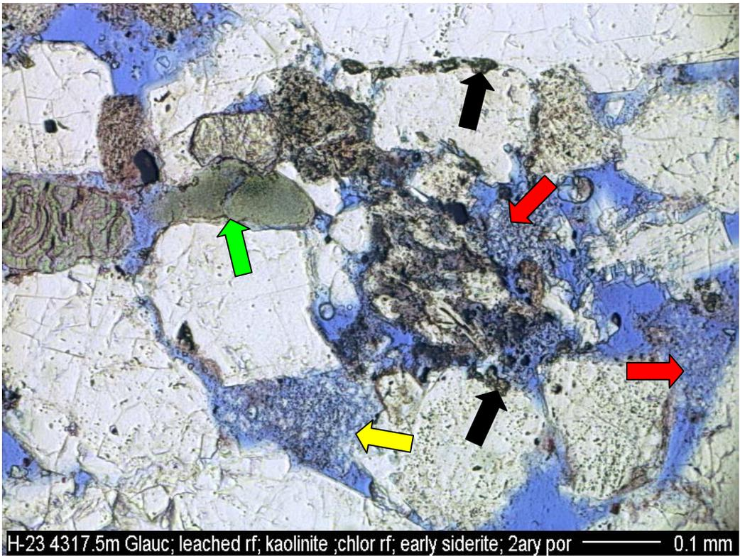
**5 and 6)** Glauconite (green arrow) is present in trace to minor amounts. Secondary porosity has formed by partial to complete dissolution of unstable rock fragments (red arrows) and feldspar (white arrow). A minor amount of early microcrystalline siderite (black arrows) clings to some grains or is compacted between grains. Kaolinite locally fills reduced primary and secondary pores (yellow arrows).
