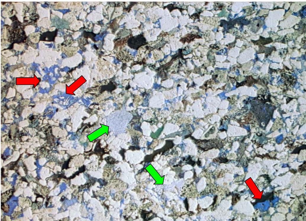
H-23 4318.5m Mw sort lvf-uf, dom lf litharenite; abun kaol; high micropor — 0.1 mm
