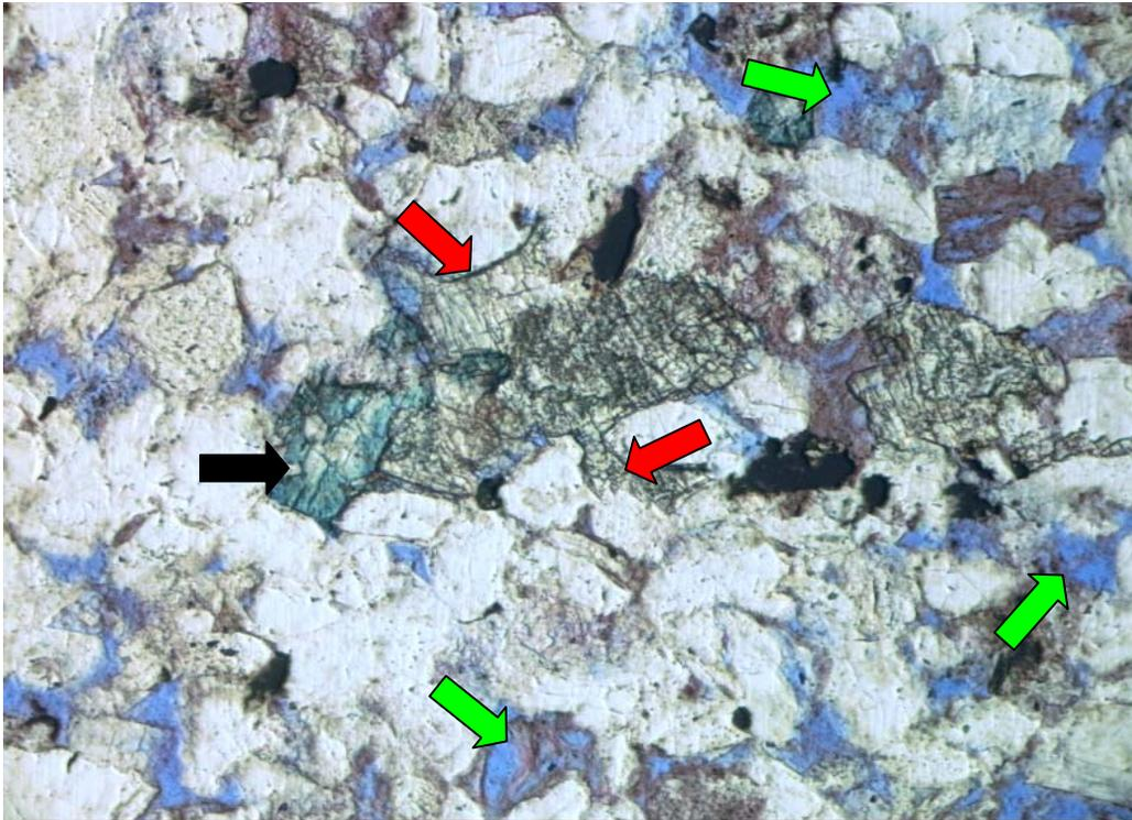
H-23 5407.5m Fecc, dol cmt; reduced intergr and 2ary pores; SiO2 cmt ——— 0.1 mm
