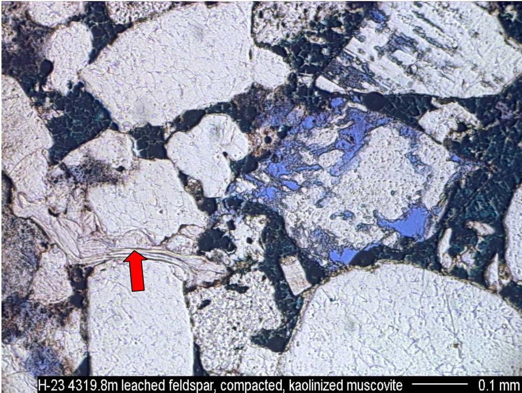
**5 and 6)** Same field of view under plane polarized light (5) and under crossed polars (6). Most porosity occurs as intragranular dissolution porosity in microcline (upper right), and other alkali feldspars (right center). A muscovite grain (red arrows) was deformed by compaction before ferroan calcite cement precipitated. Mica is partly altered to kaolinite.
