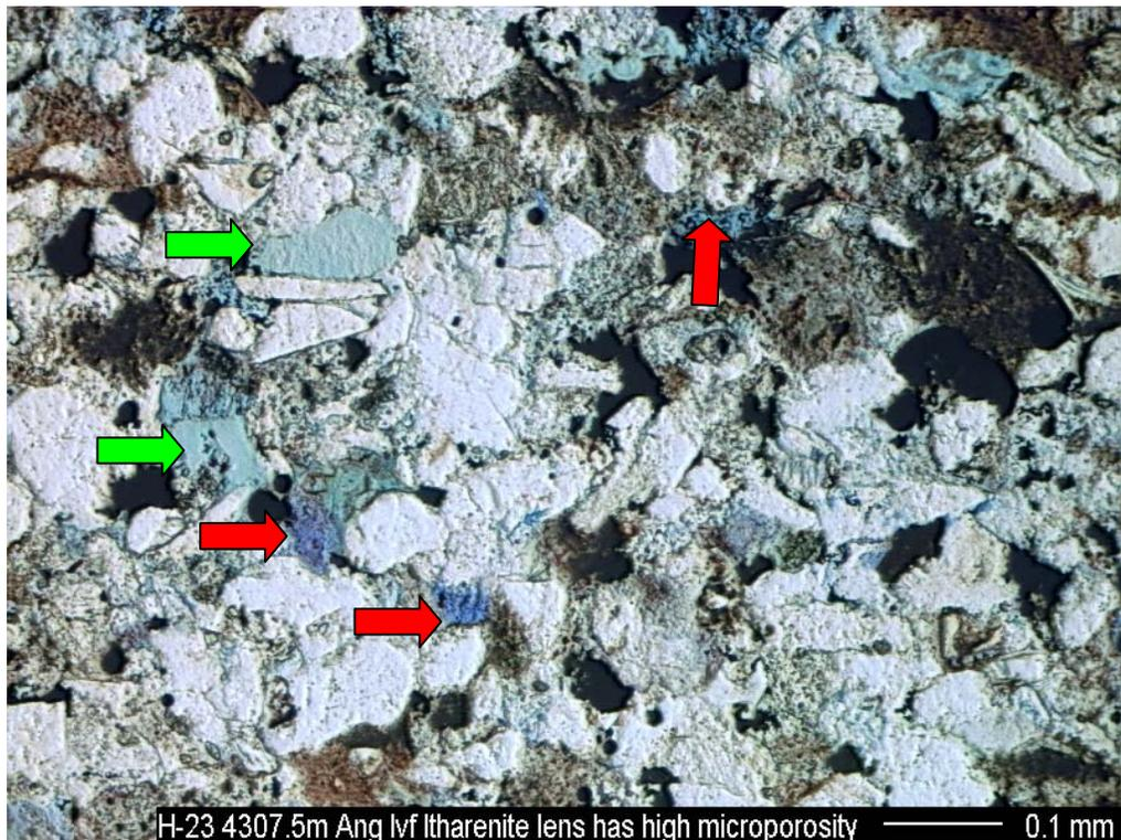
H-23 4307.5m Ang lvf litharenite lens has high microporosity — 0.1 mm
