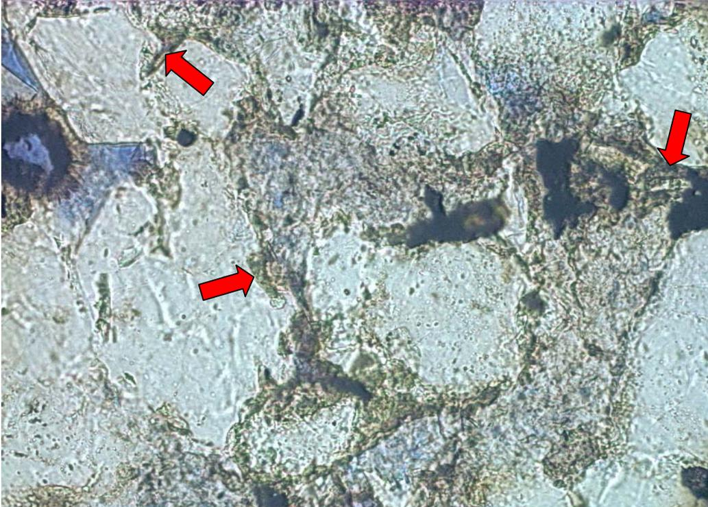
H-23 5406.5m Early chlorite rims grains; kaolinite, SiO<sub>2</sub> cmt; auth — 0.010 mm
