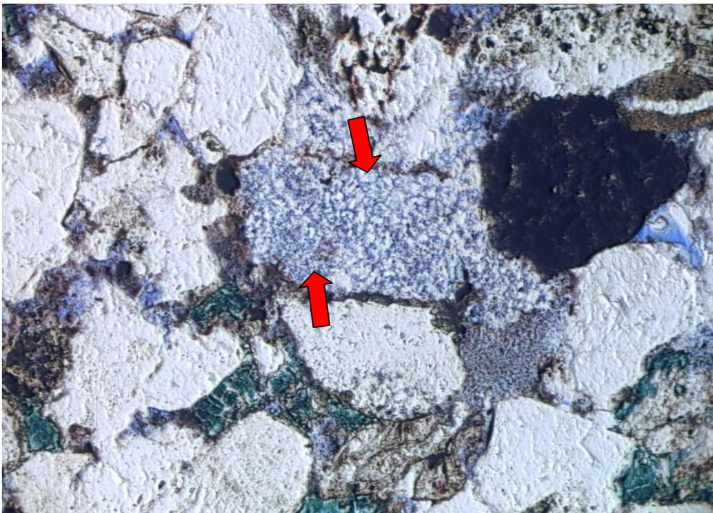
H-23 4349.7m Siderite rims on moldic pore filled by kaolinite: Fecc cmt ——— 0.1 mm
