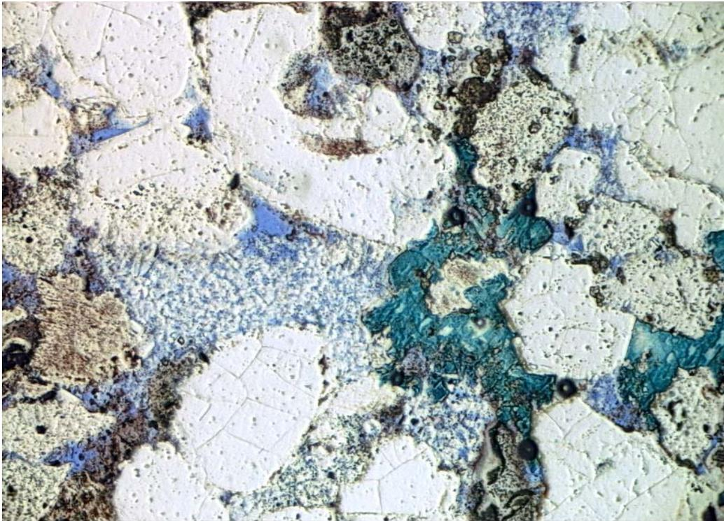
H-23 4354.5m Kaolinite in moldic pore predates SiO<sub>2</sub> and Fecc cement ——— 0.1 mm
