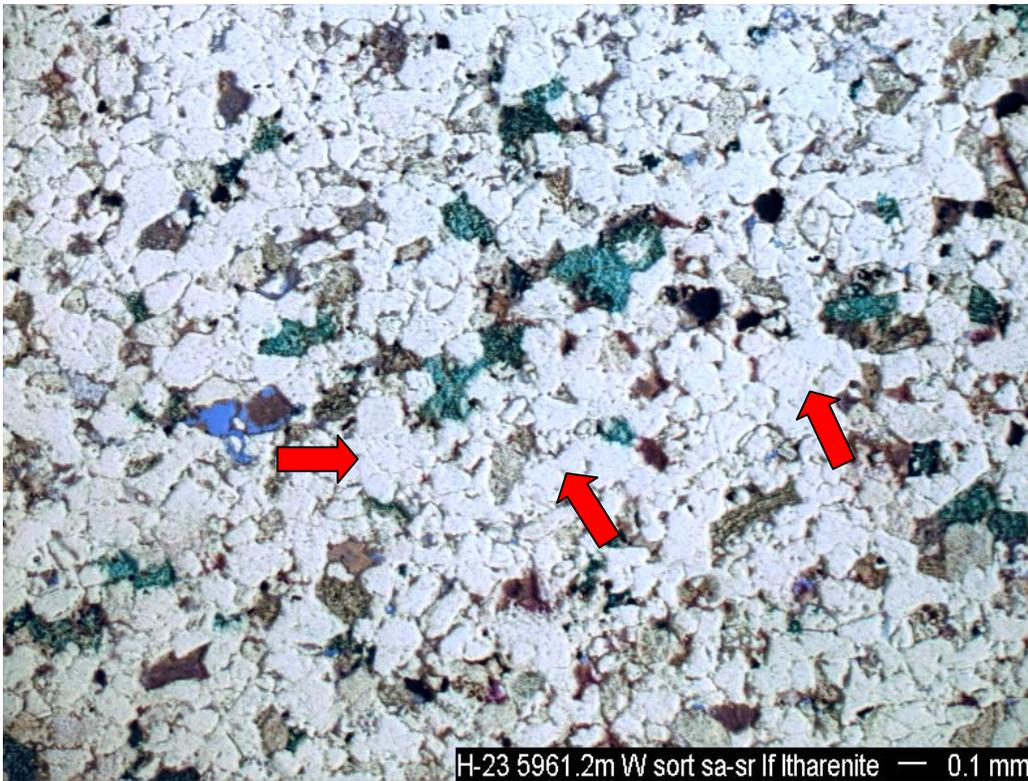
1 and 2) Well sorted subangular to subrounded lower fine grained litharenite. Intergranular porosity is almost completely occluded by close grain packing and silica cement (red arrows), scattered ferroan calcite and ferroan dolomite (blue-green). Ferroan calcite usually fills pores [black arrow, (2)] and ferroan dolomite usually partially replaces unstable clasts (green arrow). Discontinuous authigenic chlorite rims do not significantly inhibit quartz overgrowth development (blue arrows).
