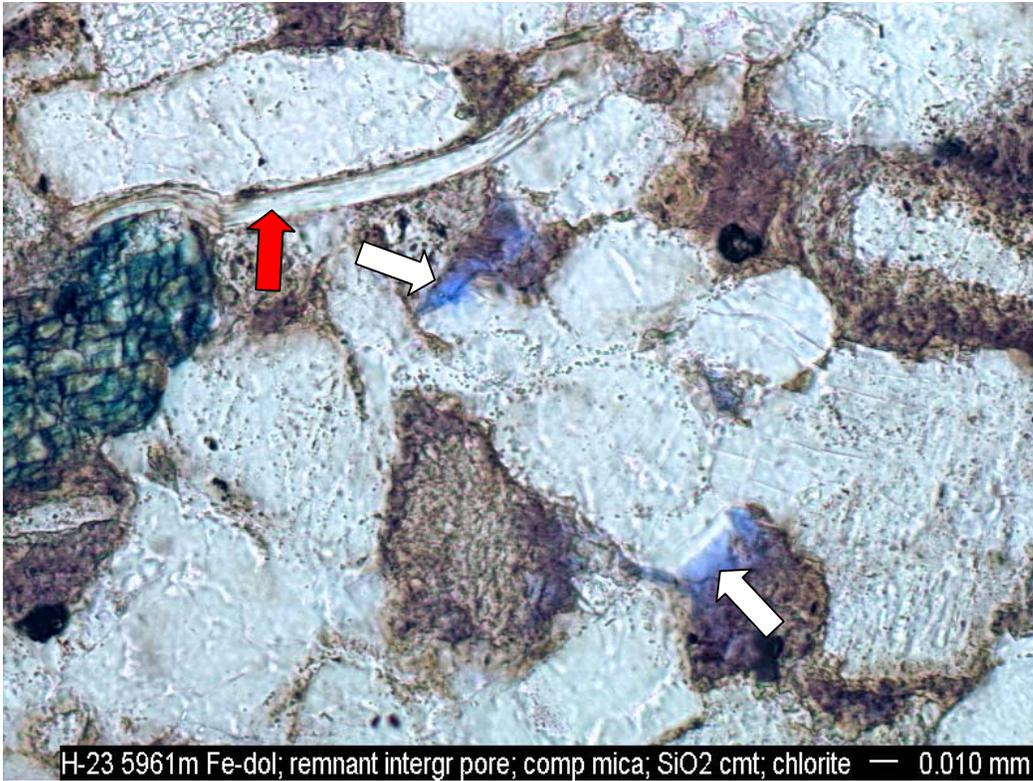
**3 and 4)** Same field of view under plane polarized light (3) and under crossed polars (4). Intergranular porosity is severely reduced by close grain packing, compaction of ductile mica (red arrows), rock fragments and interstitial clays into pores, and by silica cement. Isolated remnant reduced intergranular porosity is locally preserved (white arrows). A trace amount of moldic porosity has formed by dissolution of unstable clasts.
