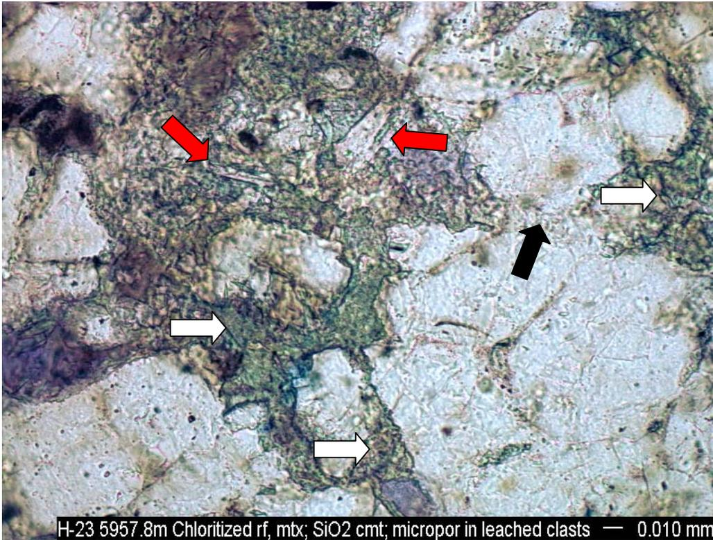
**3 and 4)** Same field of view under plane polarized light (3) and under crossed polars (4). Volcanic rock fragments (red arrows), argillaceous clasts and detrital matrix clays are chloritized (white arrows). Silica cement (black arrow) and compacted ductile clasts and matrix clays reduce intergranular porosity. Minor microporosity is present in leached clasts.
