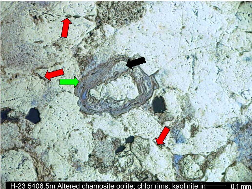
H-23 5406.5m Altered chamosite oolite; chlor rims; kaolinite in — 0.1 mm
