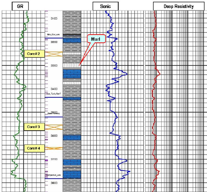
**Figure 52.** Shubenacadie H-100: Well logs from the turbidite target. The section consists of shale, limestone and marl.
