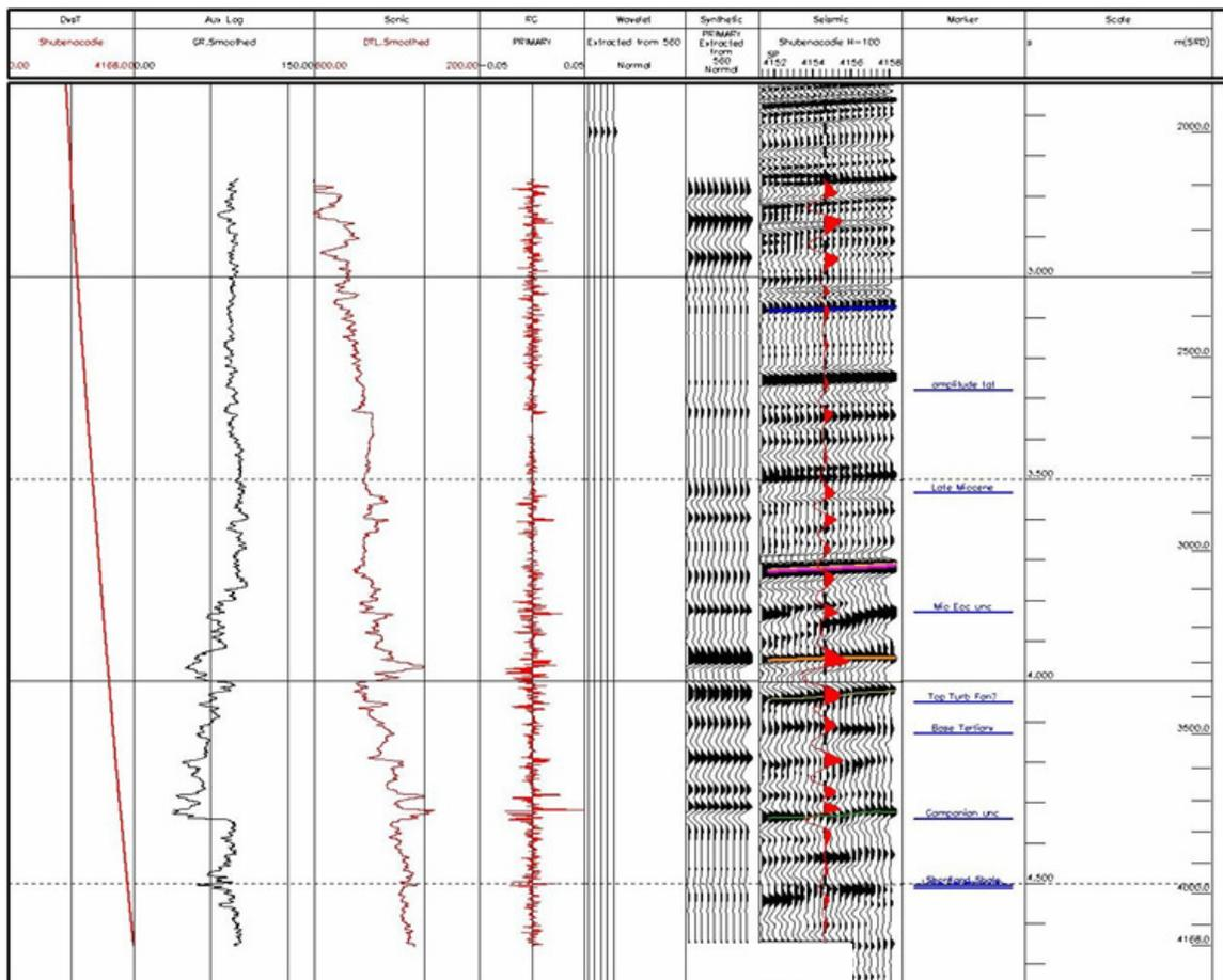
Figure 54. Shubenacadie H-100: Synthetic seismic.
