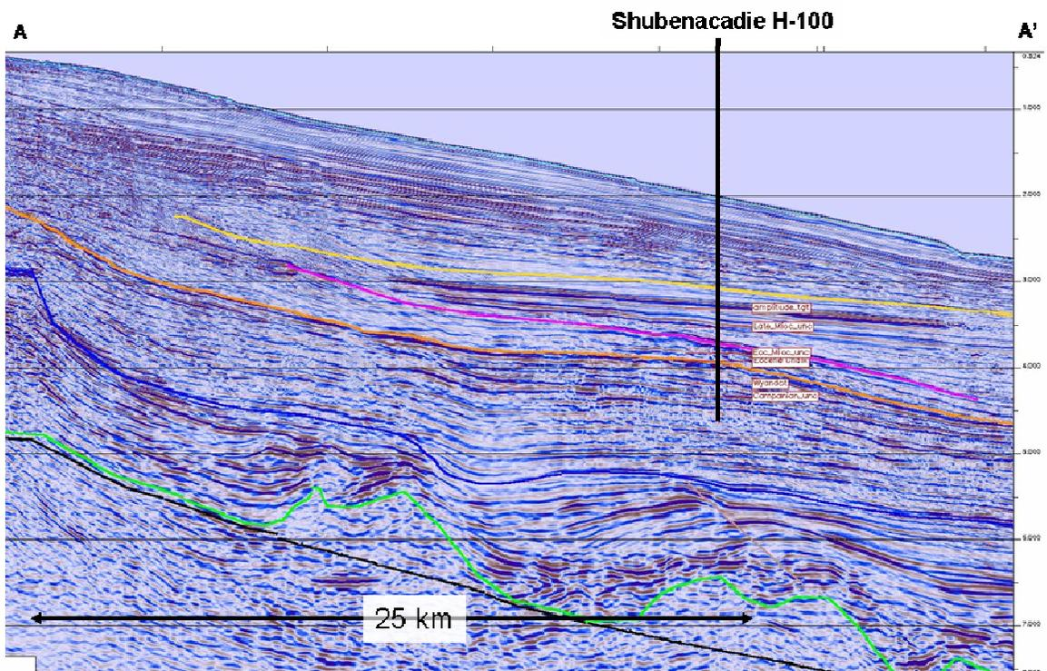
**Figure 49.** Regional 2-D seismic dip line through Shubenacadie H-100. The targets for this well included the amplitude anomaly at 2.3 seconds (TWT) and the thickened mound below the orange horizon, interpreted as a possible turbidite. Data courtesy of TGS-NOPEC.
