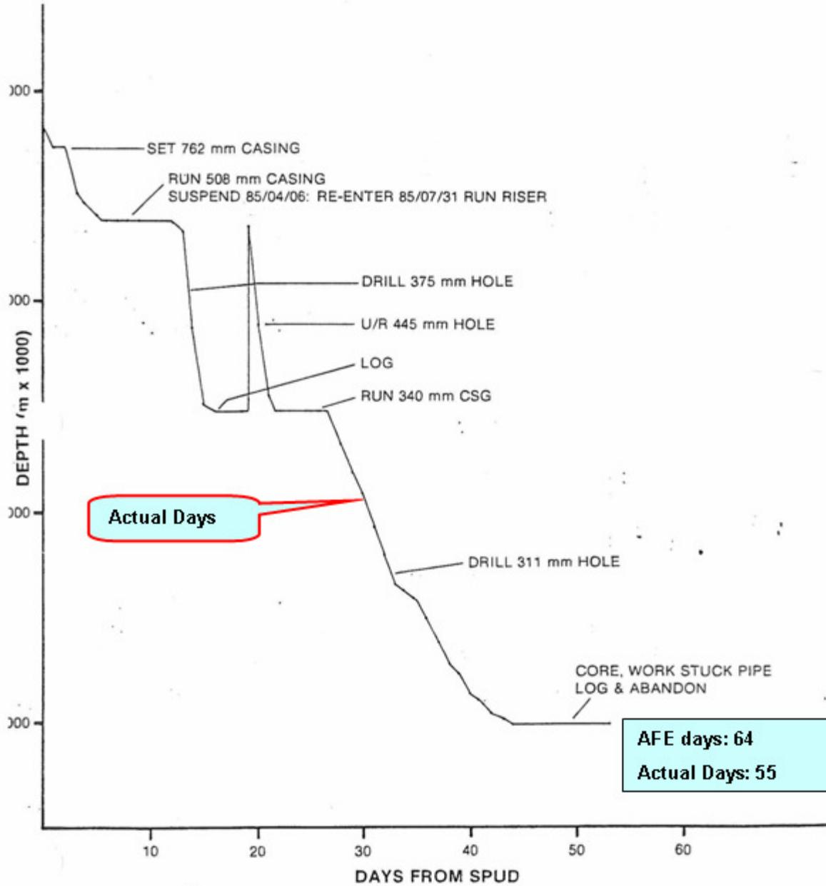
Figure 75. Shelburne G-29: Time vs. depth curve (actual).
