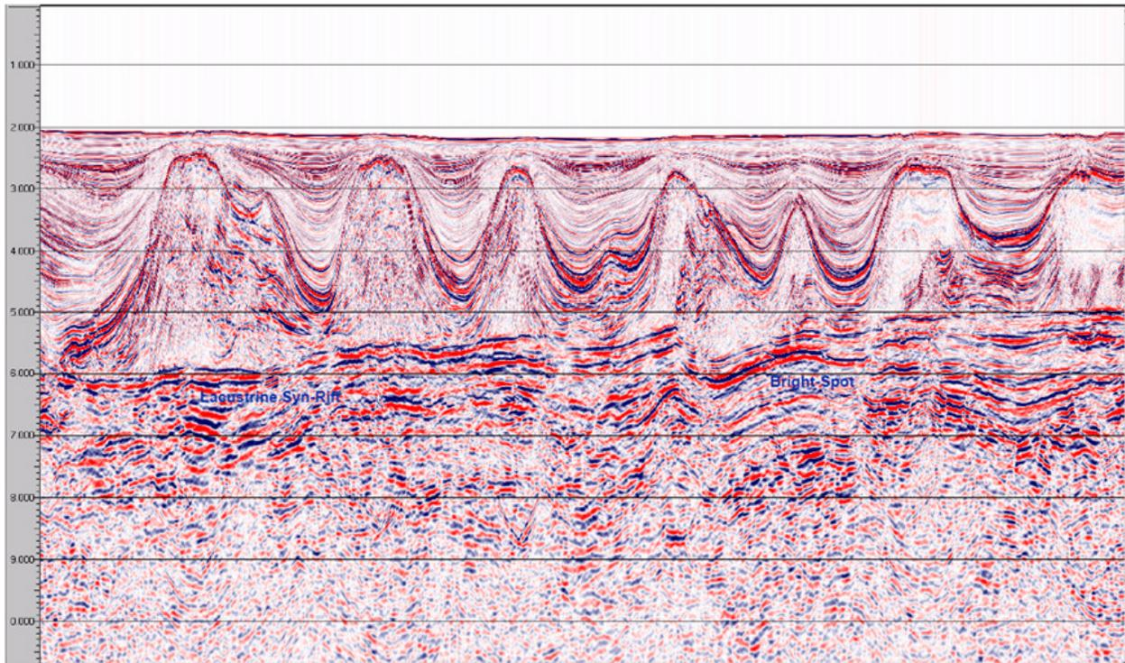
**Figure 40.** Strike seismic section from the Sao Paulo Plateau of the Santos Basin, Offshore Brazil. Bright spots indicate possible sub-salt plays, beneath the allochthonous salt canopy (Fainstein, 2003).
