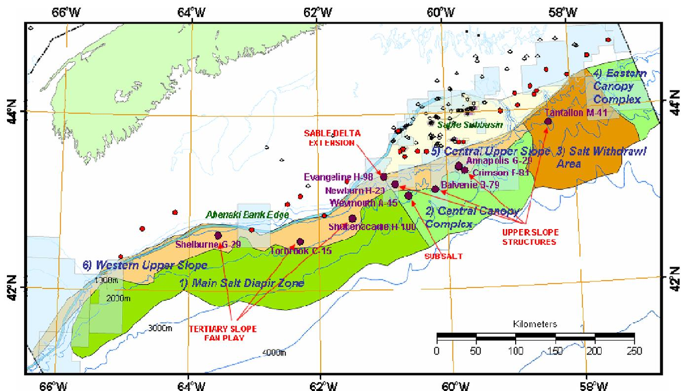
**Figure 1.** Deepwater location map. The shaded areas represent different geological provinces within the deepwater slope. The extents of the Jurassic carbonate bank and the Sable Sub-basin are also shown. Purple annotated wells were the focus of this study. The type of play tested by each well is shown in red. Transparent blue polygons show the 2006 land interests.
