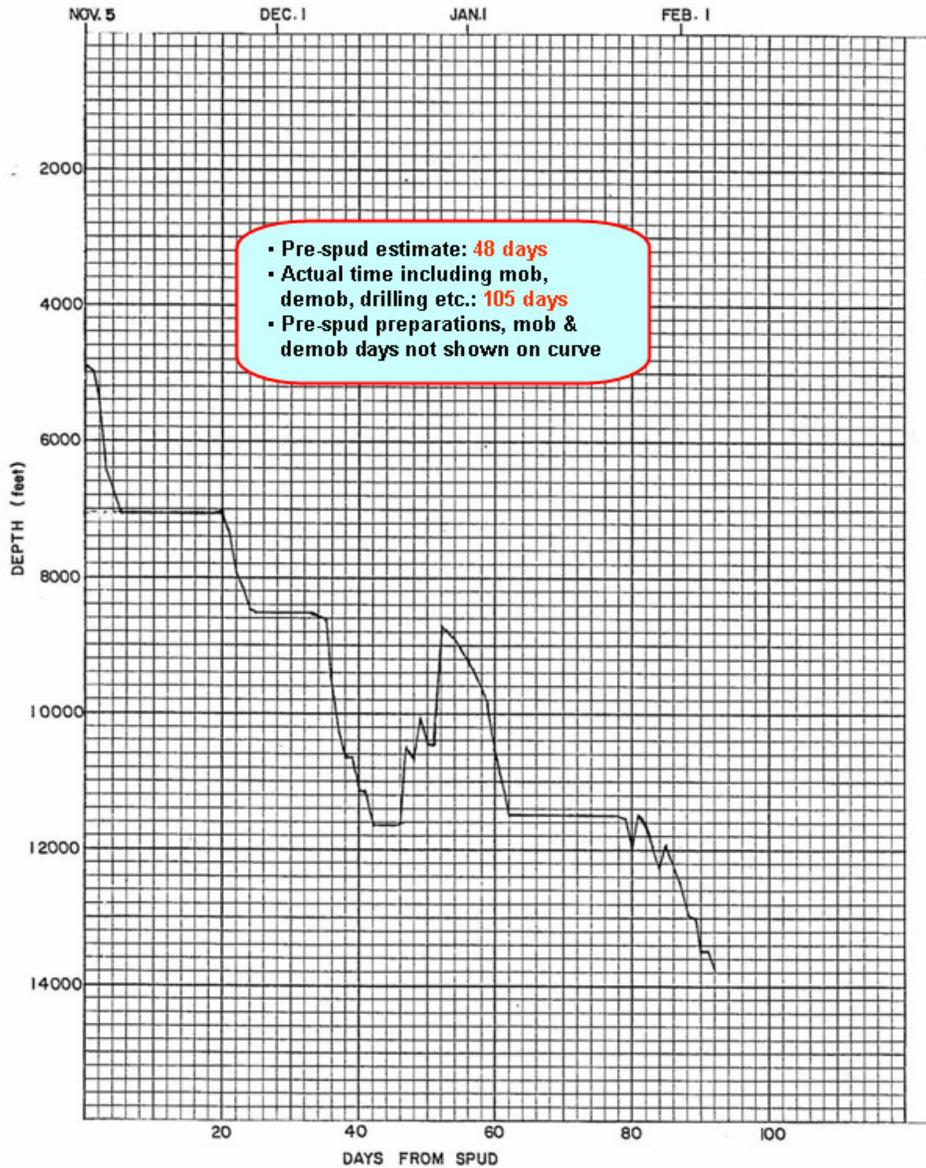
Figure 55. Shubenacadie H-100: Time vs. depth curve (actual).
