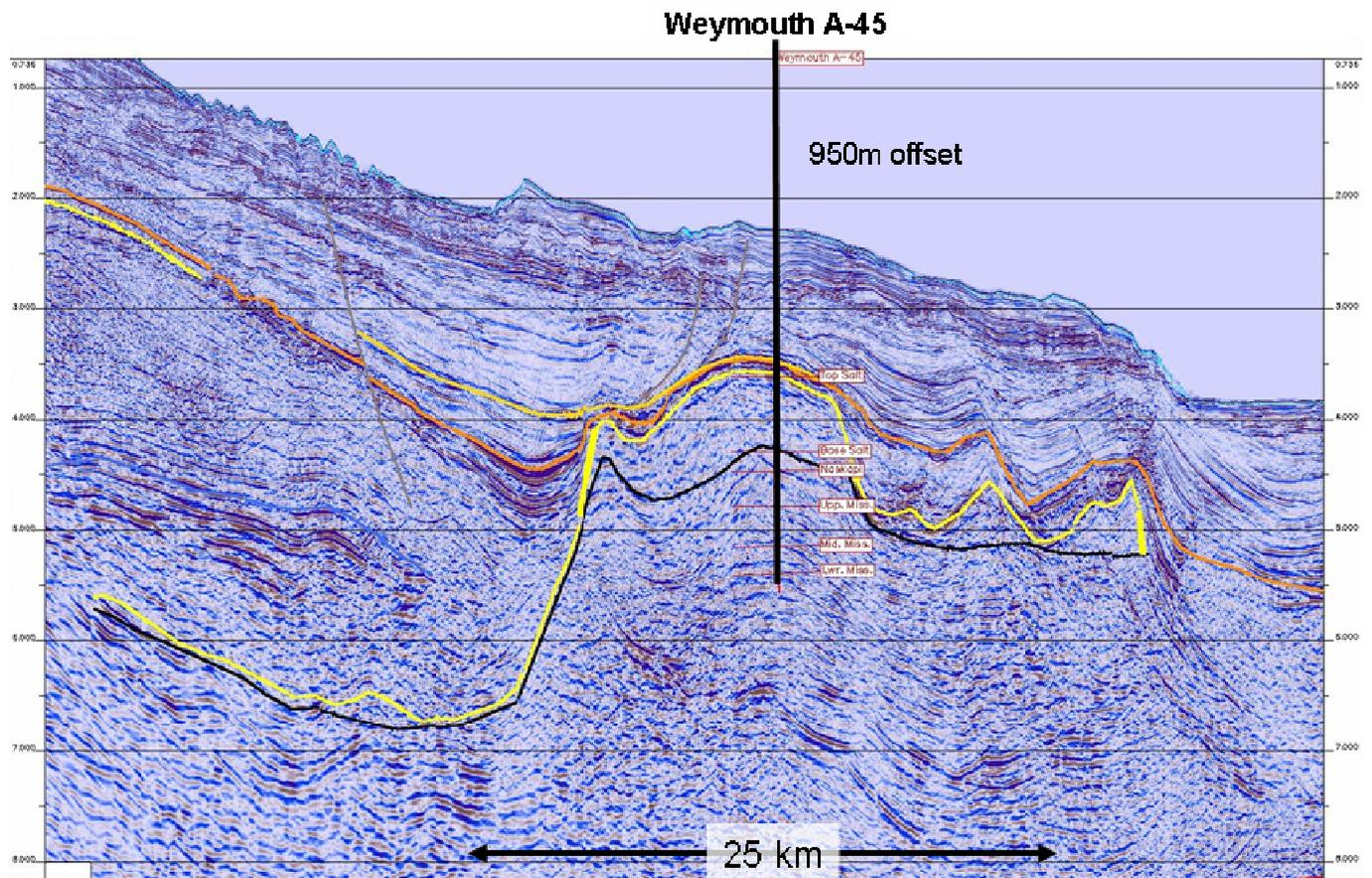
**Figure 139.** Seismic dip line (2-D) through Weymouth A-45. Black horizon is the base of the salt. Data courtesy of TGS-NOPEC.
