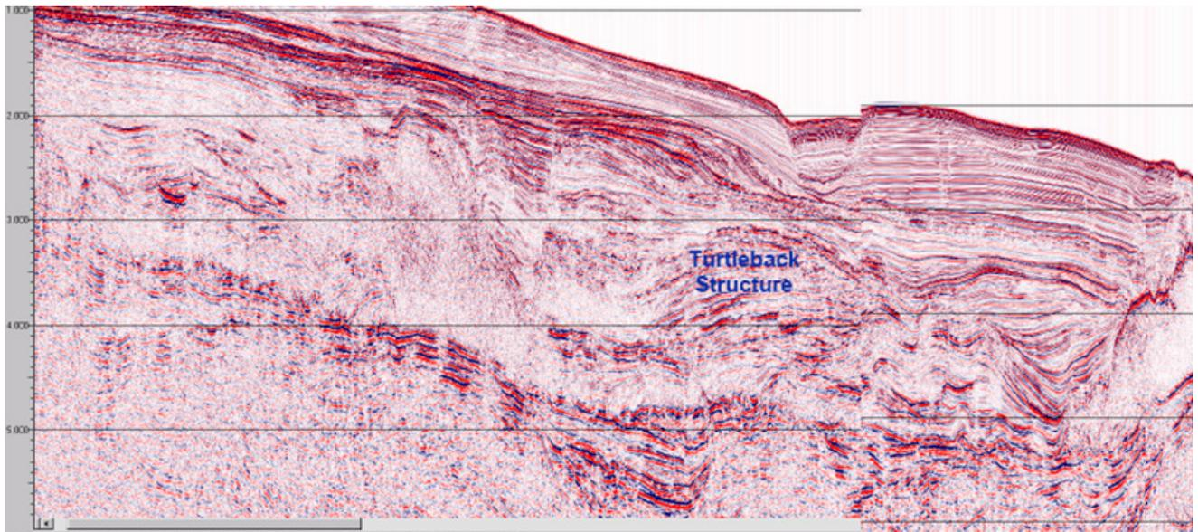
**Figure 38.** Dip seismic section from the Santos Basin, Offshore Brazil. A turtle-back structure, formed via salt withdrawl, is highlighted. Similar structures are found in the Deepwater Scotian Slope (Fainstein, 2003).
