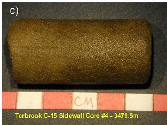
**Figure 116.** Sidewall core photos from Torbrook C-15. a) Siltstone from Tertiary 34 zone. b) Shale from Tertiary 34 zone. c) Very fine-grained sandstone from Tertiary 20.
