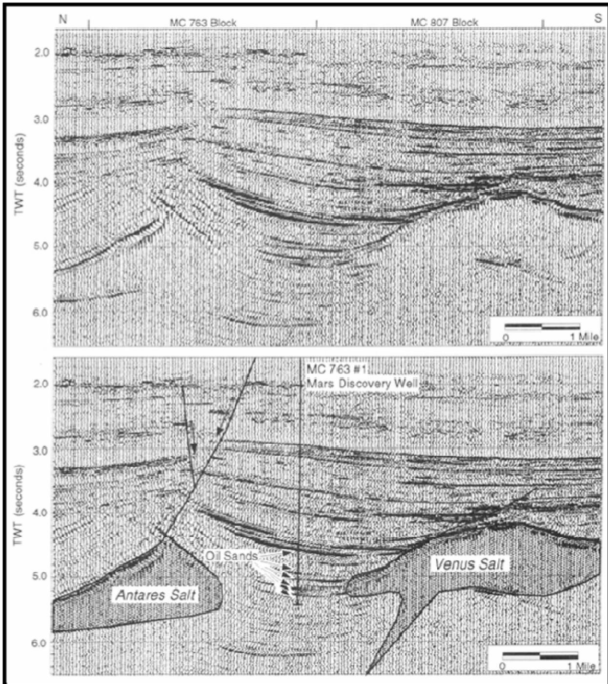
**Figure 27.** Seismic section through the Mars Field. Top is uninterpreted, bottom is interpreted. The bright amplitude anomalies between the salt bodies represent the major hydrocarbon-bearing sands (Mahaffie, 1994).
