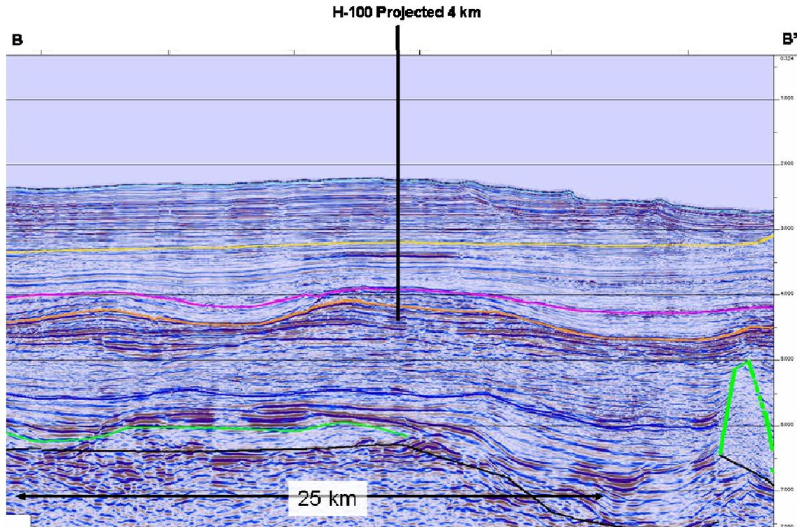
**Figure 50.** Regional 2-D seismic strike line near Shubenacadie H-100. The deeper target (orange) is an erosional remnant, bounded by two channels in this view, not a mounded turbidite deposit. Data courtesy of TGS-NOPEC.
