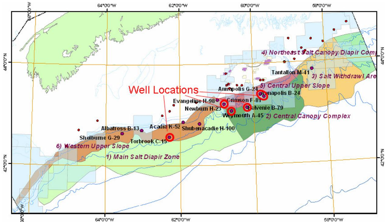
**Figure 174.** Deep-water map showing the subsurface geologic zones. The plays recalculated after recent drilling are restricted to zones 2, 5, and 6, as they are the only zones with recent wells (red circles).
