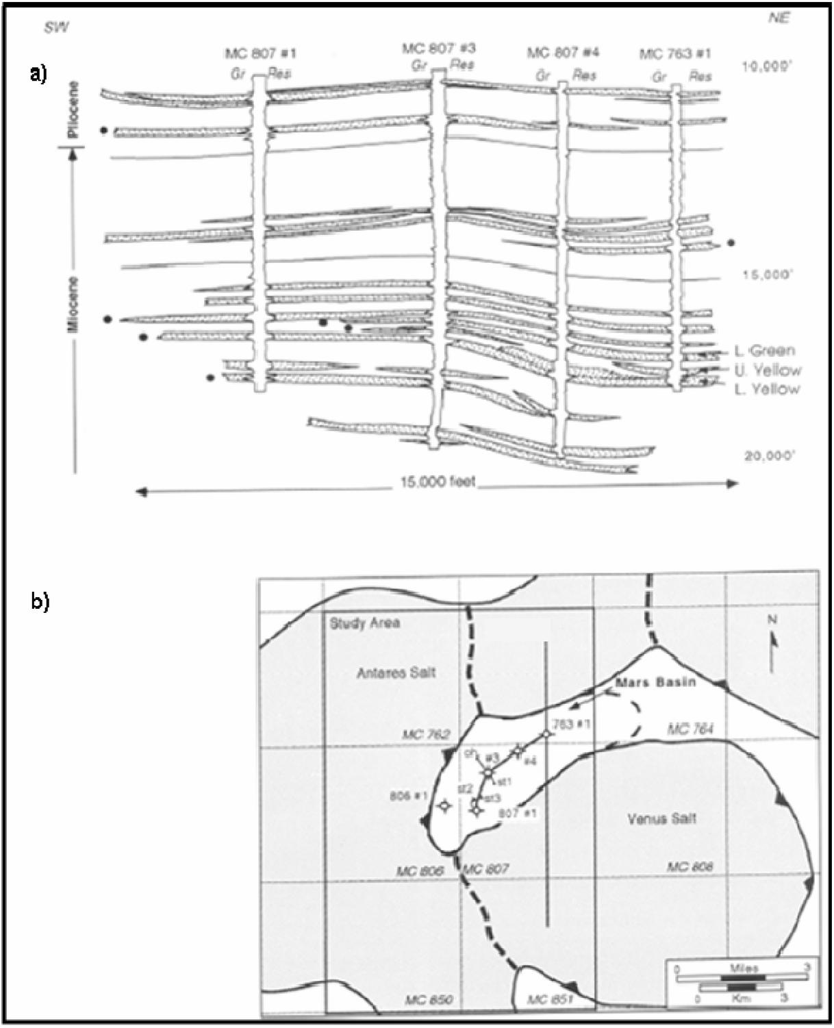
**Figure 26.** a) Correlation section through the Mars Basin, illustrating the distribution of turbidite sands encountered. Black circles indicate reservoir. b) Base map for the Mars Basin. The black line connecting the wells is the cross-section shown in (a). The vertical line indicates the location of the seismic section shown in Figure 24 (Mahaffie, 1994).
