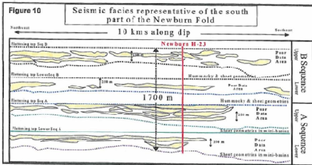
Figure 100. 3-D seismic dip section and interpreted facies for Newburn H-23, from the Newburn H-23 ADW (used with permission).
