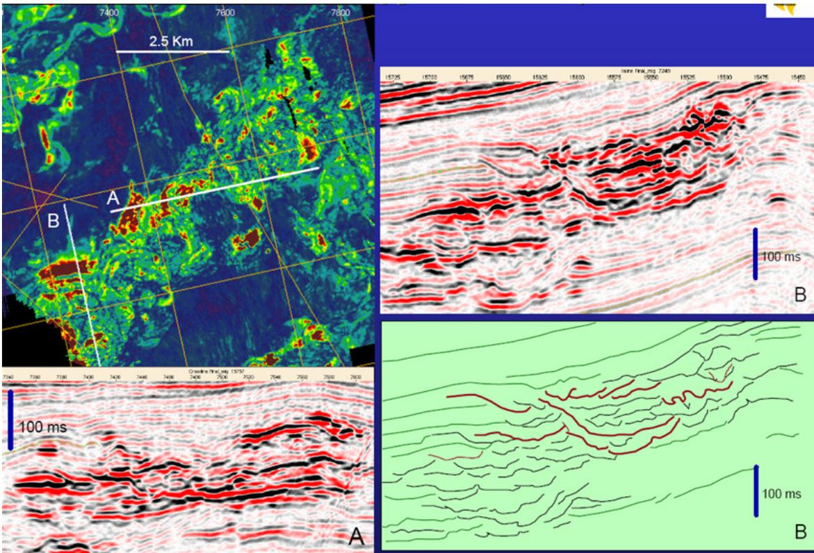
**Figure 43.** Seismic examples from a deepwater turbidite channel system, in the Lower Congo Basin. This channel system displays complex erosional features and stacked channel sequences (Gjelberg, 2003).
