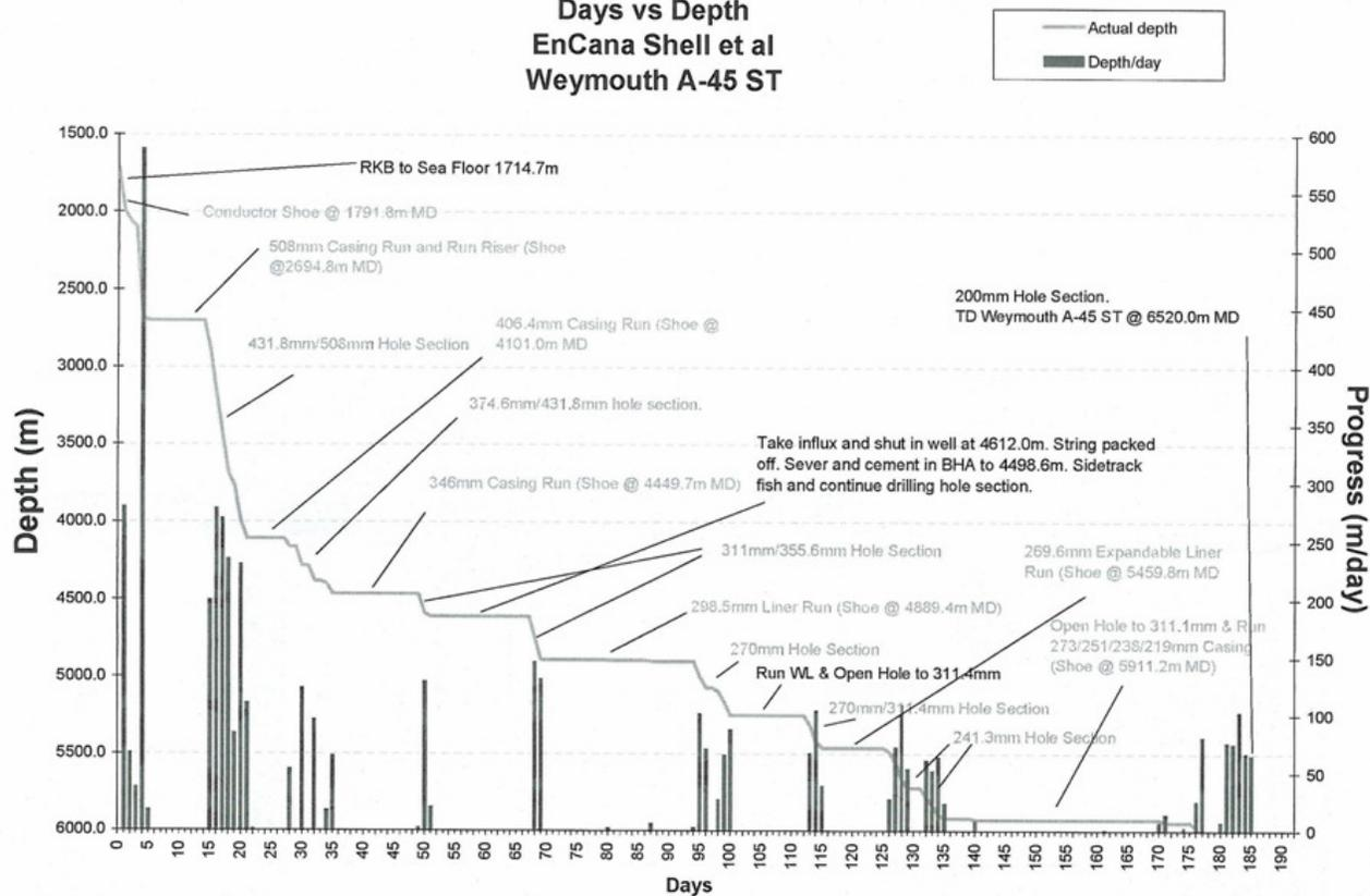
Figure 141. Drilling curve for Weymouth A-45 (actual).
