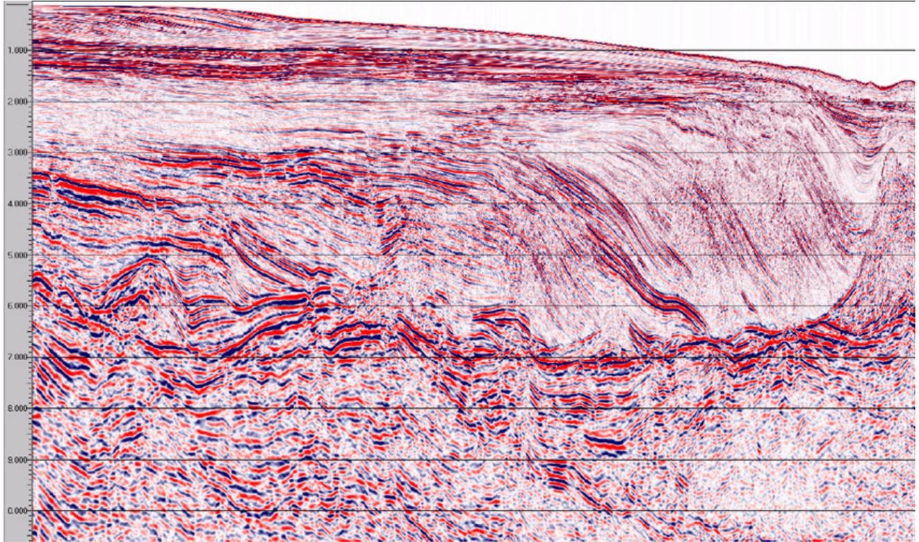
**Figure 37.** Dip seismic section from the Santos Basin, Offshore Brazil. The structures seen are similar to those of the “Salt Withdrawl” area in the Deepwater Scotian Slope (Fainstein,2003).
