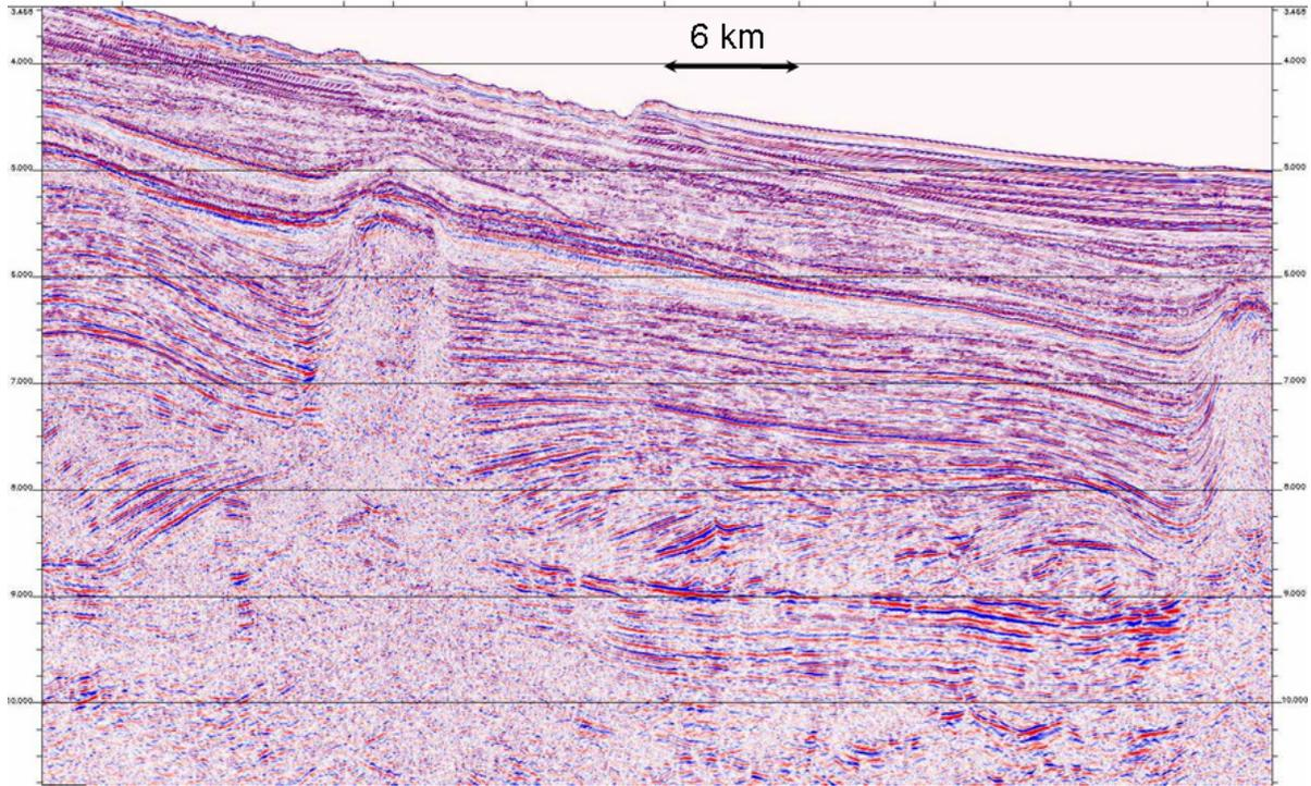
**Figure 171.** 2-D seismic example of salt rollers, from the salt withdrawl area (area 3 - Figure 1). Data courtesy of TGS-NOPEC.
