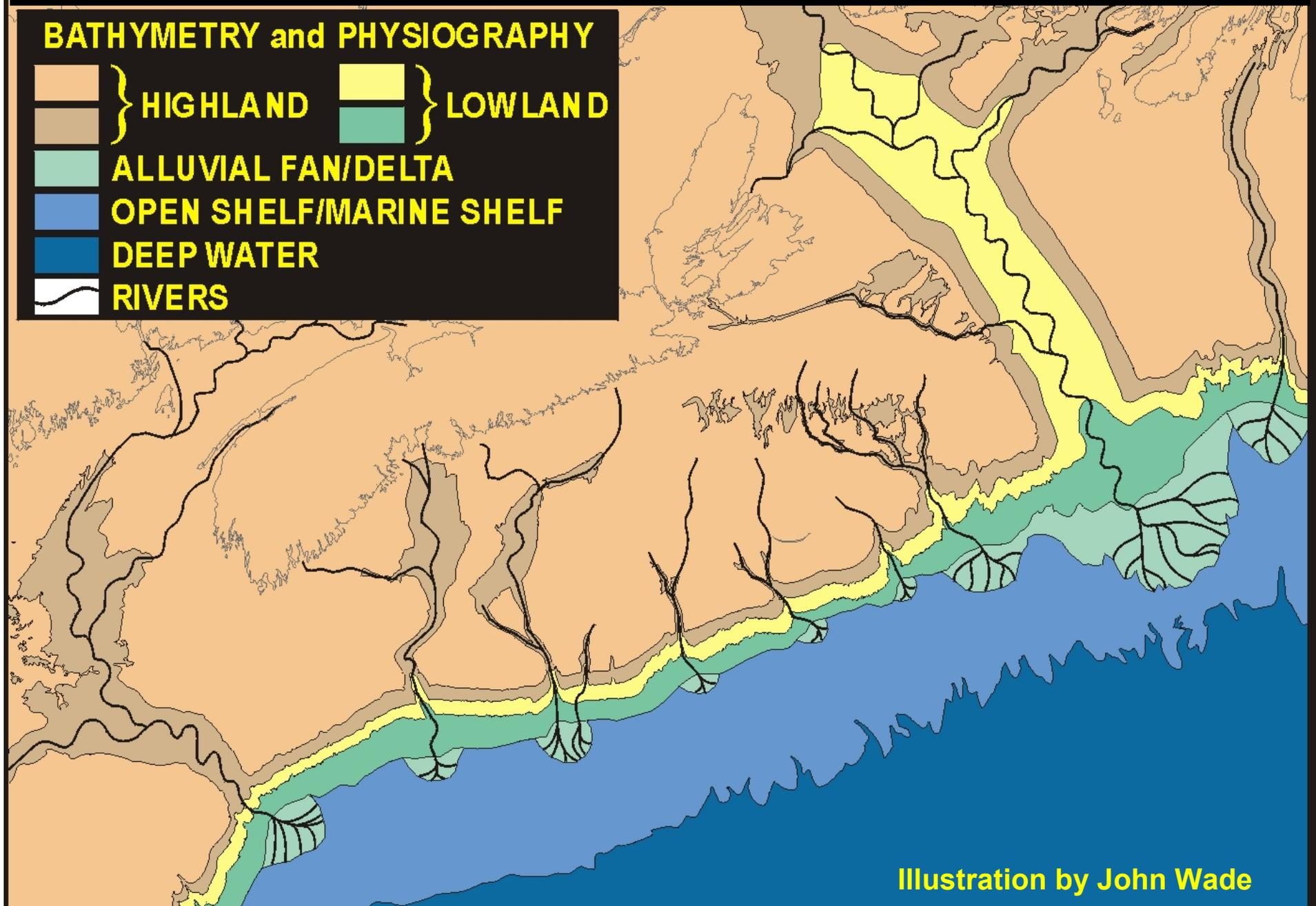
Figure 8: Simplified paleogeographic reconstruction of the Scotian Basin during the Upper Oligocene (Chattian) ca. 30 mya. The figure illustrates the Chattian age sea level fall and resultant exposure and erosion on the Nova Scotia margin (Chattian unconformity). Smaller shelf margin deltas and their locations are speculative. Slightly modified after the Atlantic Geoscience Society - Copyright © AGS – used with permission.
