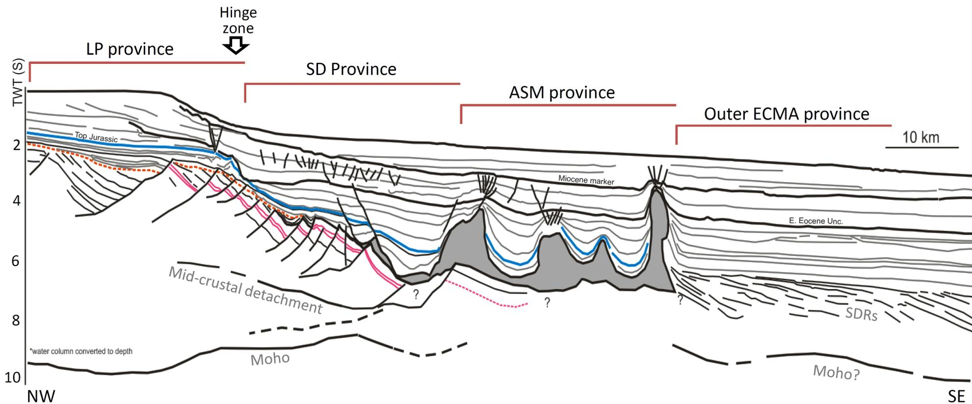
**Figure 2** – Line drawing of a composite seismic profile extending from the LaHave Platform (LP), across the Slope Detachment (SD) and Allochthonous Salt and Minibasin (ASM) provinces, and terminating in the Outer ECMA province where Seaward Dipping Reflections (SDRs) are recognized. Water column was depth converted, but remaining section is in two-way travel time. See Figure 1a for location.
