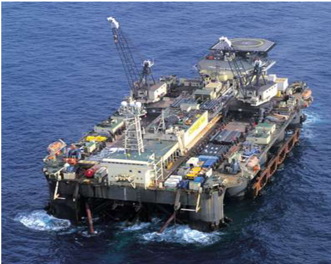
Figure 5.1 Typical Pipelaying Vessel – Castoro SEI
