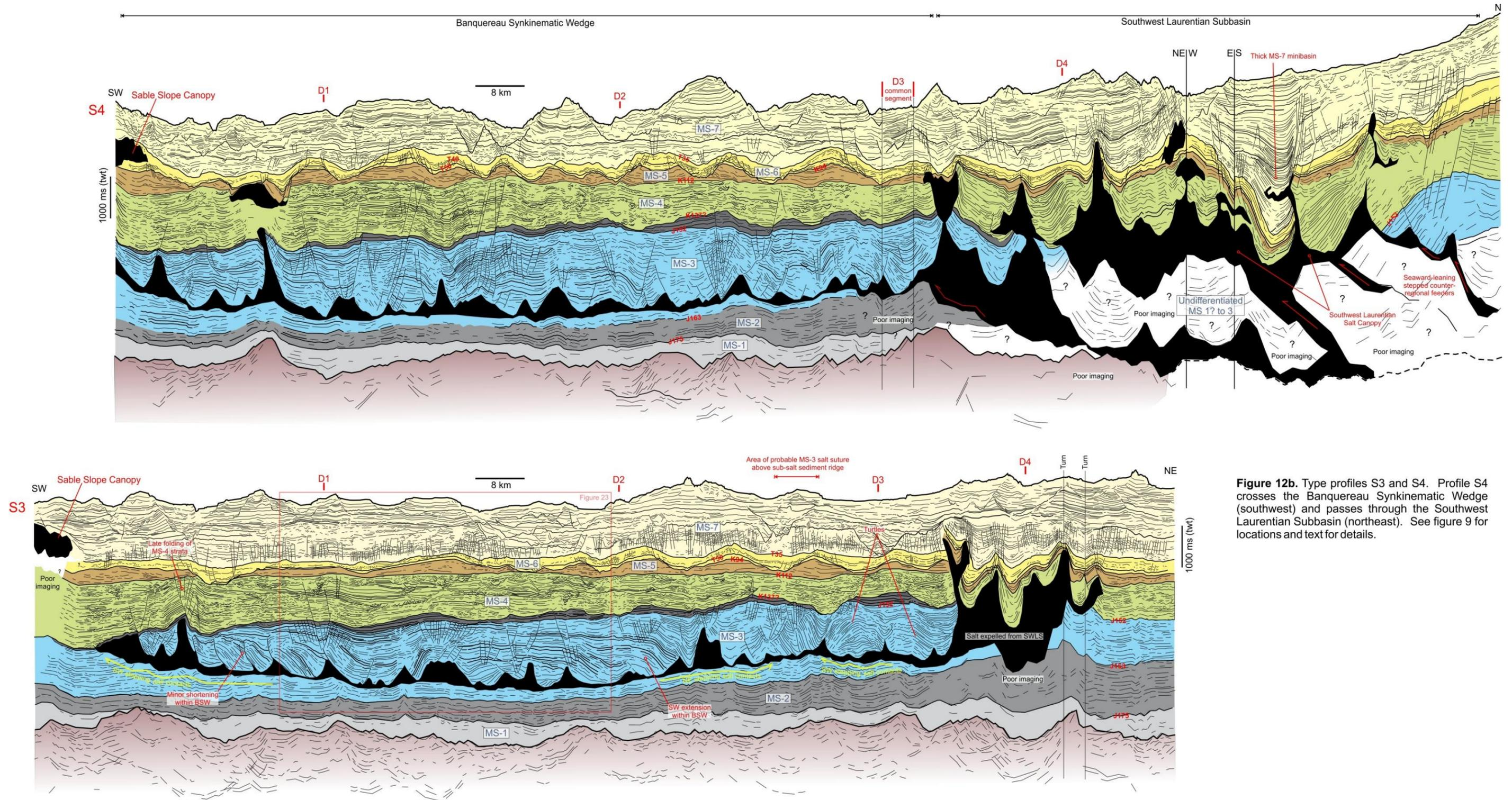
**Figure 12b.** Type profiles S3 and S4. Profile S4 crosses the Banquereau Synkinematic Wedge (southwest) and passes through the Southwest Laurentian Subbasin (northeast). See figure 9 for locations and text for details.
