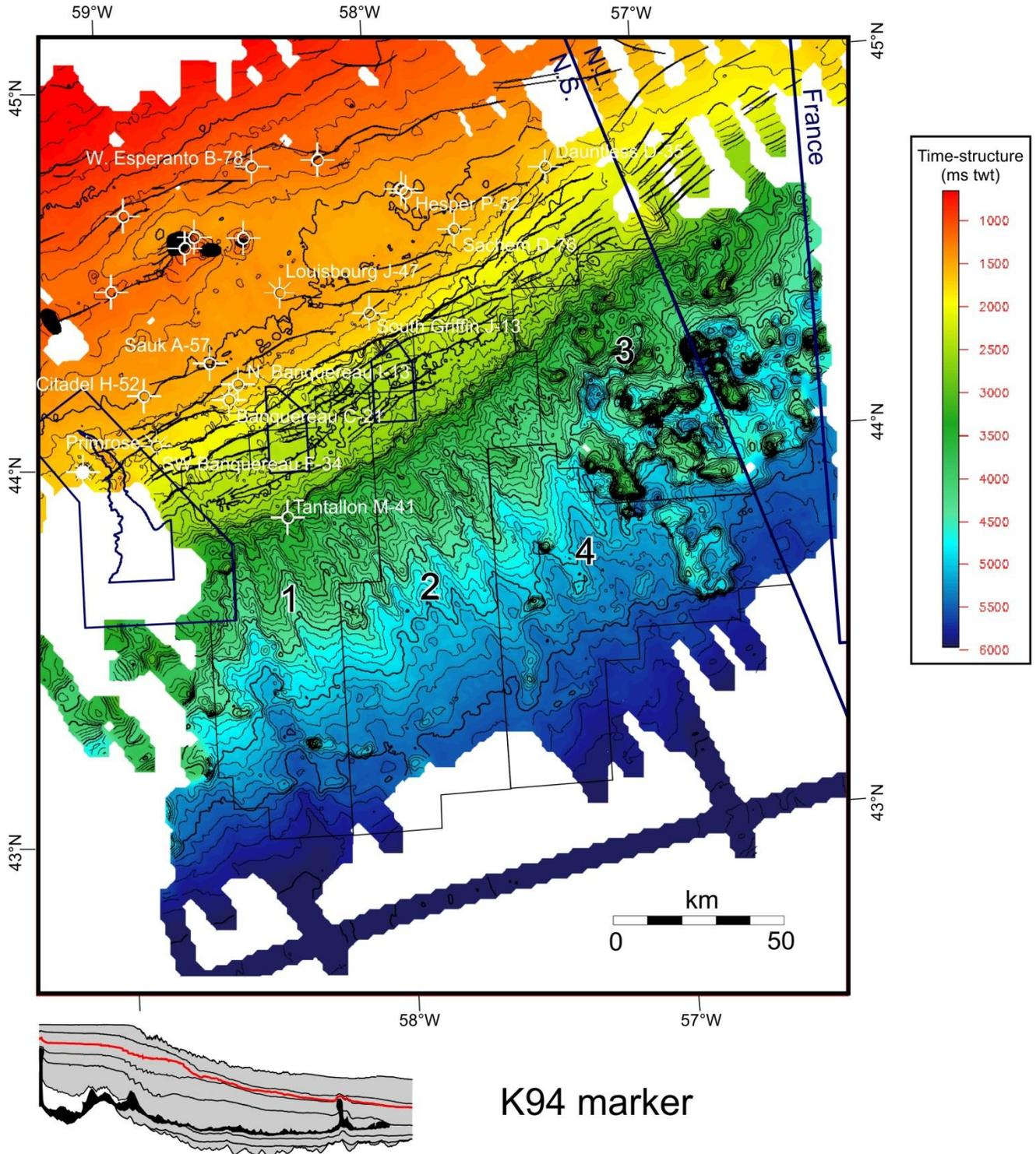
Figure 26. Gridded time-structure map of the K94 marker (near base Petrel marker).
