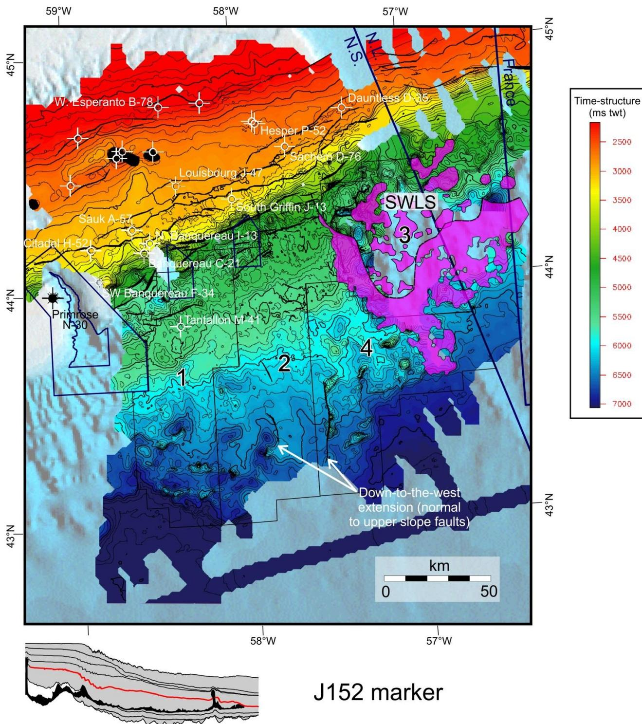
**Figure 20.** Gridded time-structure map of the J152 marker that defines the boundary between MS-3 and MS-4. Normal faults are identified in black.
