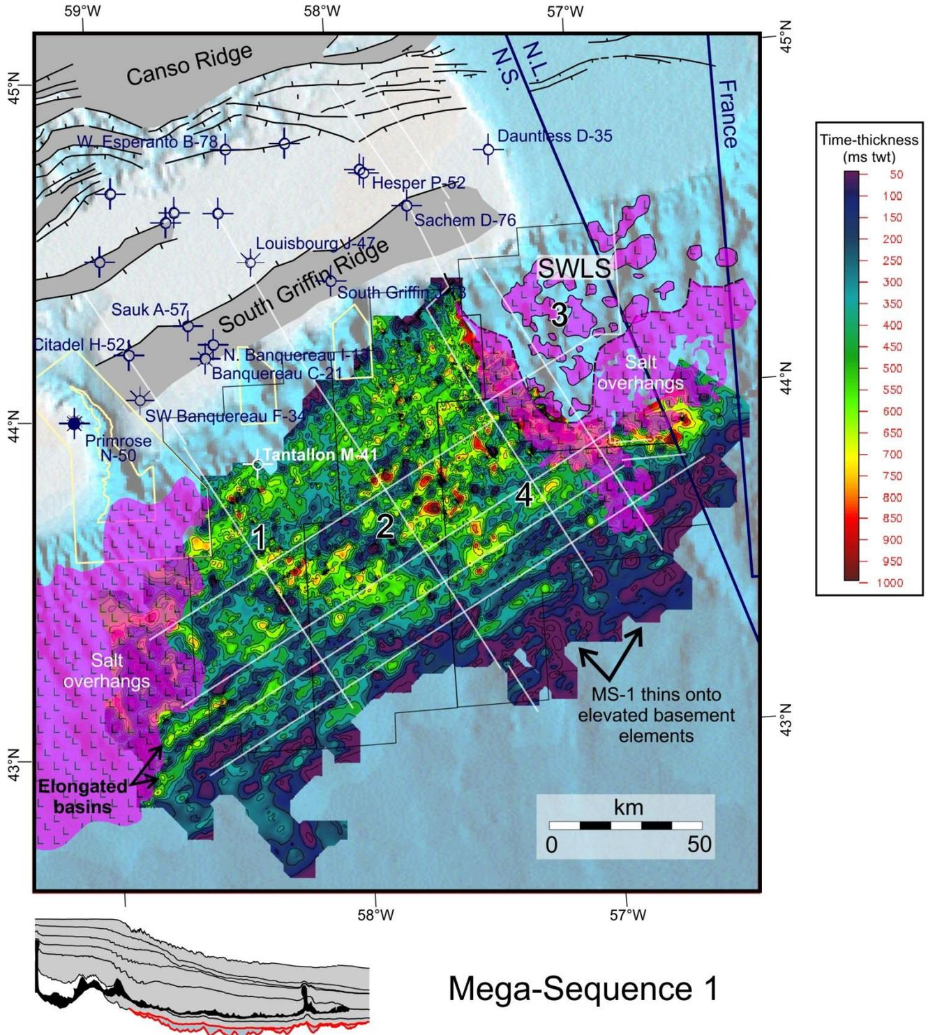
**Figure 14.** Gridded time-thickness map of Mega-sequence 1. Note the northeastern trending thicker basins that follow the trend of basement troughs between prominent basement highs. Pink overlay identifies areas of thicker overhanging salt. See text for details.
