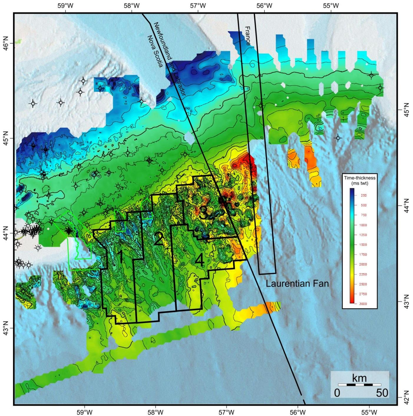
**Figure 7.** Time-thickness map between the K94 marker and the seafloor, showing the distribution of Turonian to Holocene strata. The succession corresponds closely to mega-sequences 6 and 7. See text for details.
