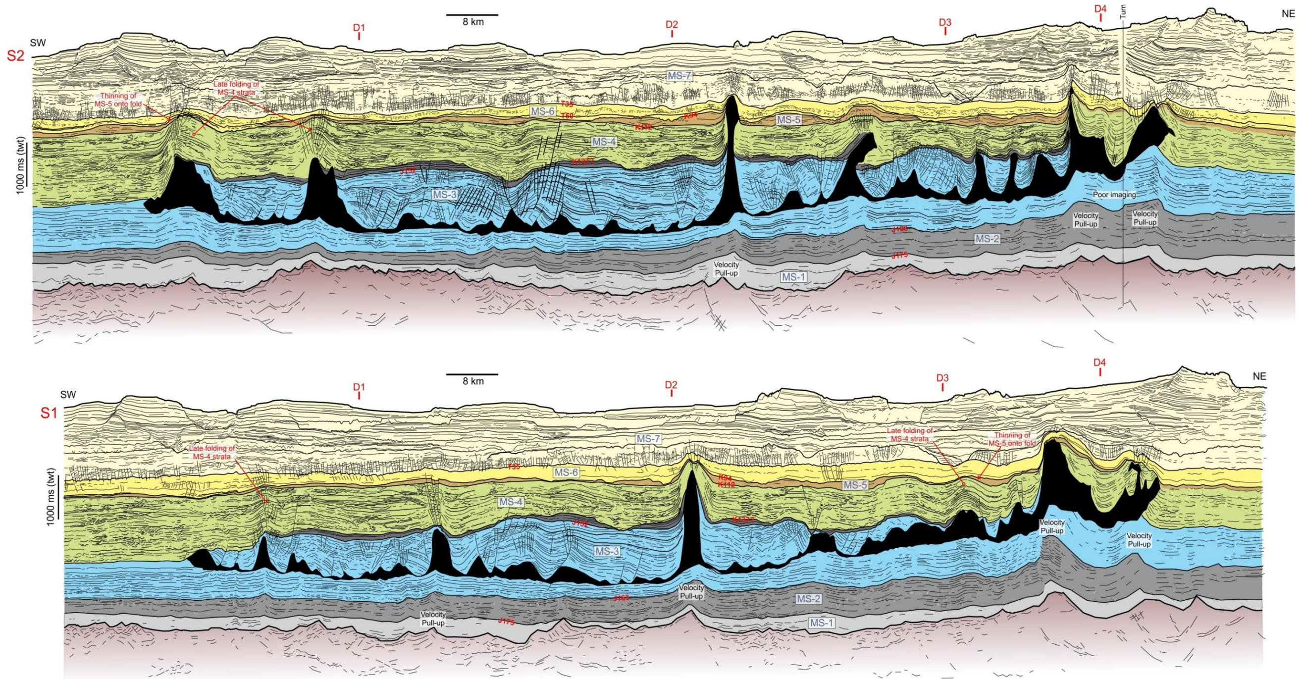
Figure 12a. Type profiles (strike-lines) S1 and S2 across the Banquereau Synkinematic Wedge. See figure 9 for locations and text for details.
