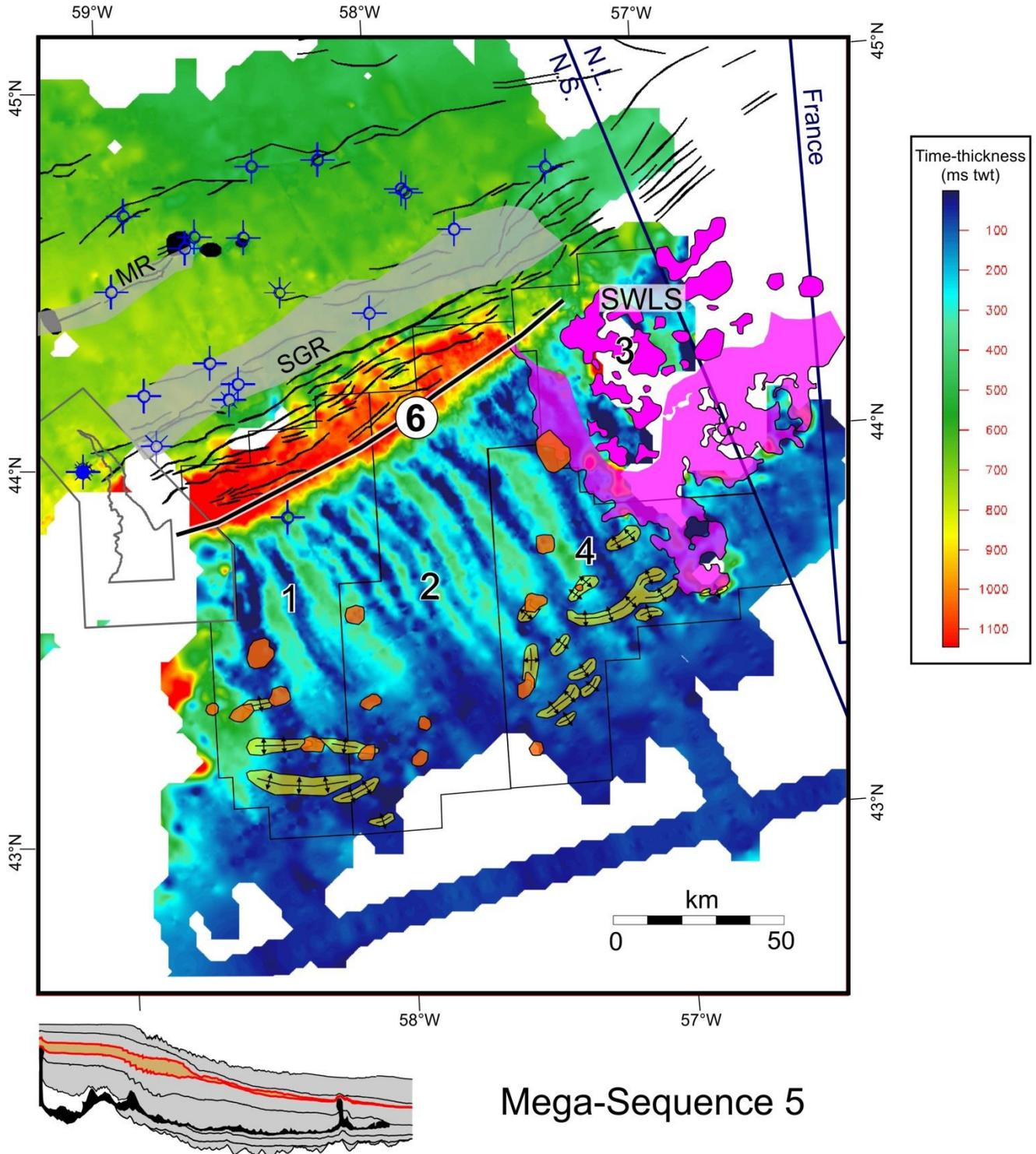
**Figure 25.** Annotated time-thickness map of Mega-sequence 5 overlain by listric normal faults on the outer shelf and showing the location of salt-cored folds along the toe of the Banquereau Synkinematic Wedge. The folds grew during MS-5, inverting turbidite-bearing strata of MS-4 (Missisauga fan complex). The distribution of pierced salt diapirs is shown in orange. Shelf-edge trajectory 6 represents the maximum regression of the margin. See text for details.
