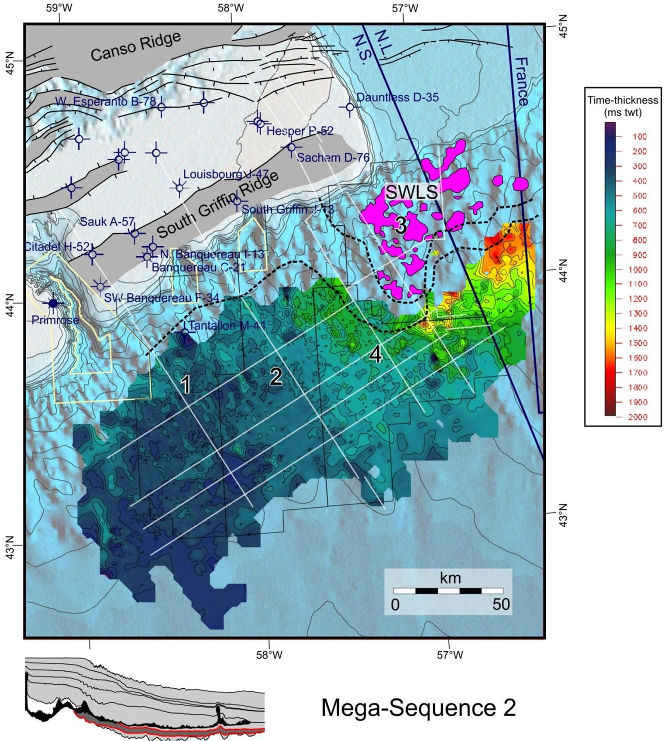
**Figure 15.** Gridded time-thickness map of Mega-sequence 2 (Middle(?) Jurassic). Note the overall decrease in thickness away from the southwestern Laurentian Subbasins (SWLS). MS-2 records the first pulse of clastics to build out towards the eastern Scotian Slope. Dashed lines identify the J175 and J163 salt contacts. See text for details.
