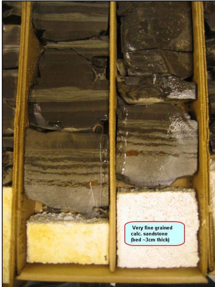
Figure 9. Tantallon M-41: Enlarged view of sandy intervals in Core #3 at ~5300 m.
