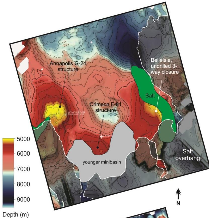
**Figure 3.1.4 a)** Depth-structure map generated on a seismic horizon near the top of the 'M' sand (~K132, late Hauterivian) intersected at the Annapolis G-24 well. Green polygons represent salt bodies, transparent black polygons are areas with salt overhang and the grey polygon is a region where the surface comes into contact with a younger minibasin (a salt body during the Hauterivian)
