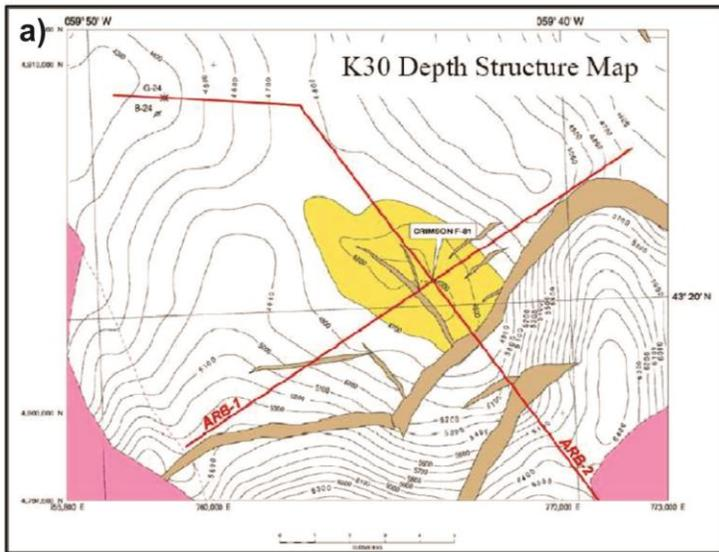
**Figure 3.1.3 a)** Pre-drill depth-structure map of Marathon's Early Aptian K30 seismic horizon at the Crimson F-81 well location. **b)** Seismic profile intersecting the Crimson F-81 well. (Both images modified after Kidston et al., 2007)
