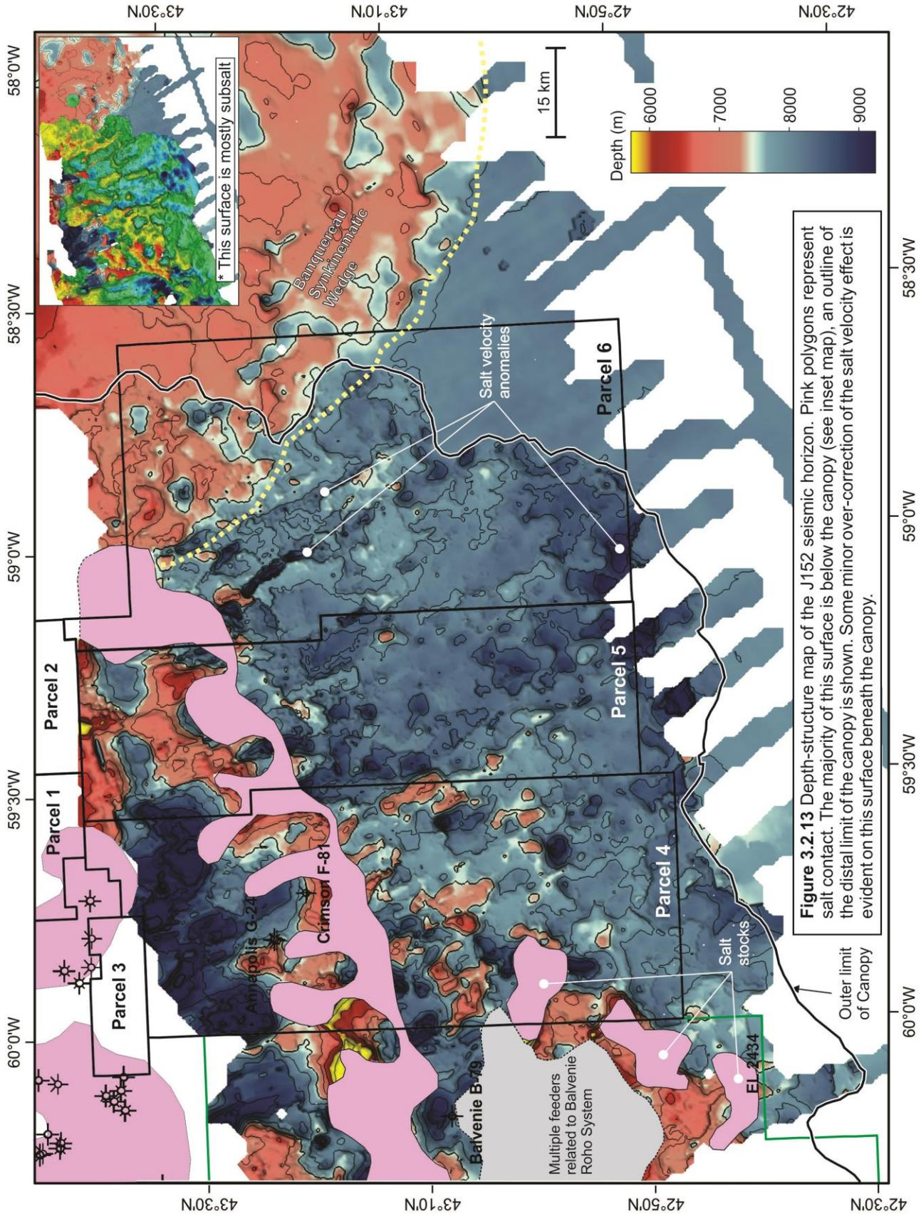
**Figure 3.2.13** Depth-structure map of the J152 seismic horizon. Pink polygons represent salt contact. The majority of this surface is below the canopy (see inset map), an outline of the distal limit of the canopy is shown. Some minor over-correction of the salt velocity effect is evident on this surface beneath the canopy.
