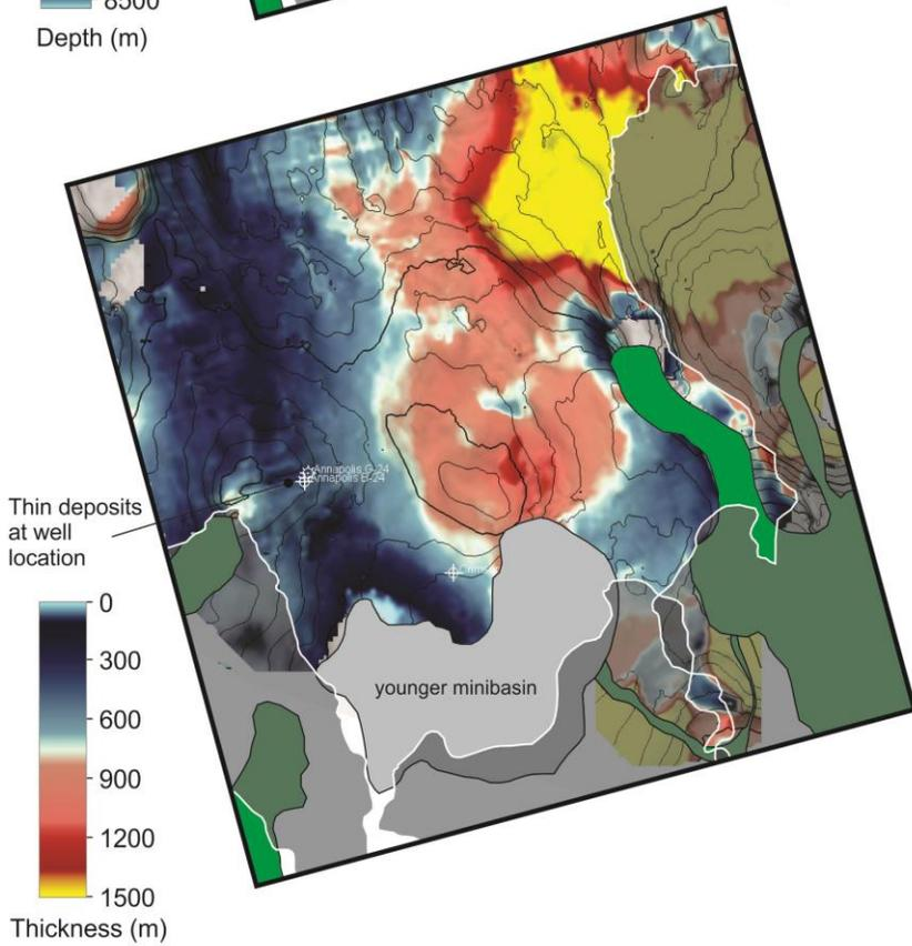
**Figure 3.1.5 b)** Thickness map between the K130 and K132 seismic horizons (Hauterivian). Depth-structure contours from the above figure. Green polygons represent salt bodies, transparent black polygons are areas with salt overhang and the grey polygon is a region where the surface comes into contact with a younger minibasin (a salt body during the Barremian)
