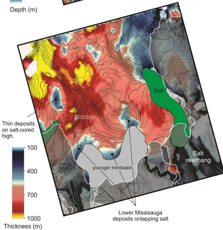
**Figure 3.1.4 b)** Thickness map between late Hauterivian (above) and top Jurassic seismic horizons, representing the thickness of the lower Missisauga (~K132 to J150). Depth-structure contours from the K132 map in 3.1.4a. Green polygons represent salt bodies, transparent black polygons are areas with salt overhang and the grey polygon is a region where the interval comes into contact with a younger minibasin (a salt body during the early Cretaceous)
