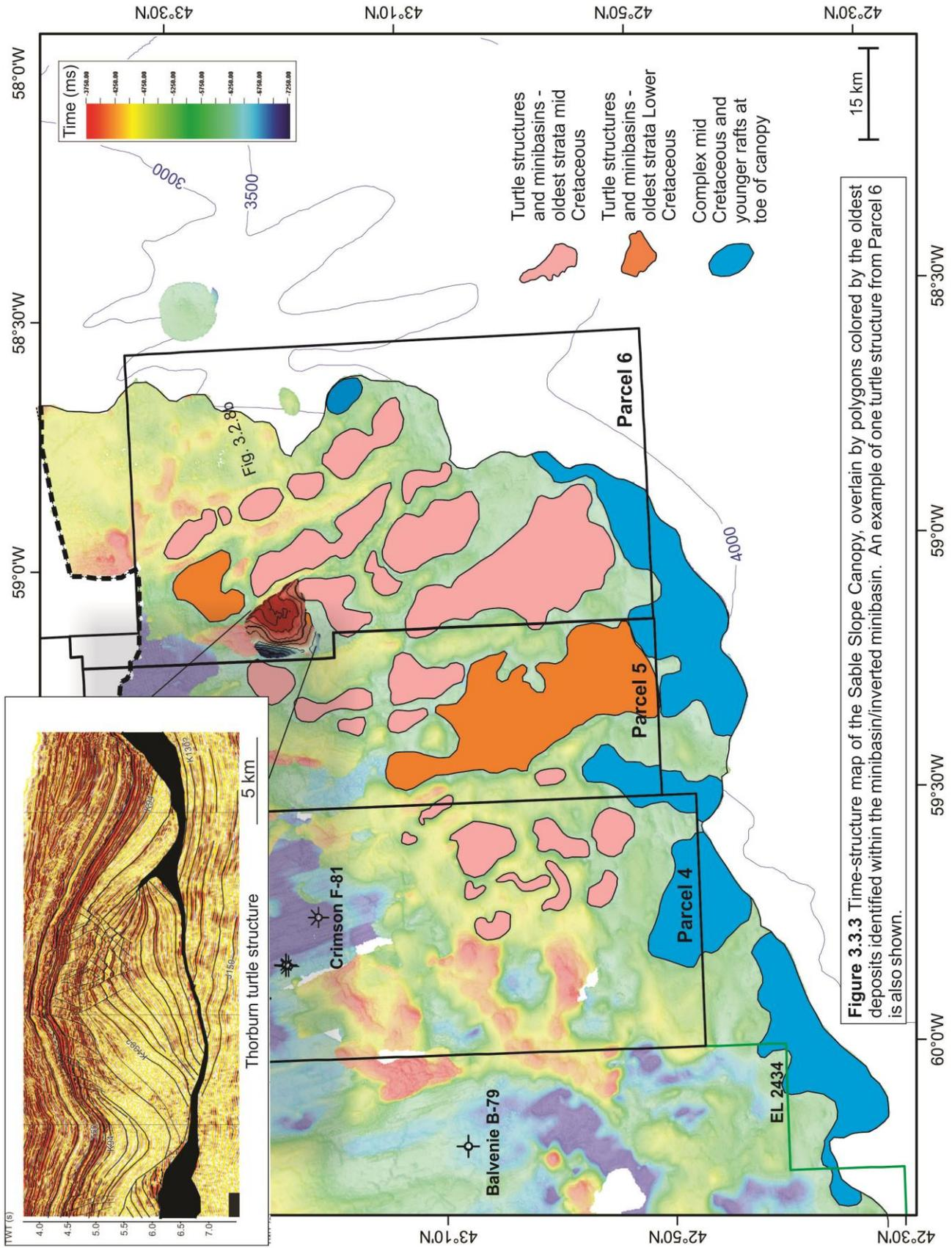
**Figure 3.3.3** Time-structure map of the Sable Slope Canopy, overlain by polygons colored by the oldest deposits identified within the minibasin/inverted minibasin. An example of one turtle structure from Parcel 6 is also shown.
