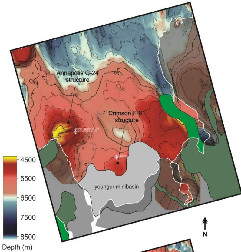
**Figure 3.1.5 a)** Depth-structure map generated on a seismic horizon near the top of the 'L' sand interval (K130, mid Barremian) intersected at the Annapolis G-24 well. Green polygons represent salt bodies, transparent black polygons are areas with salt overhang and the grey polygon is a region where the surface comes into contact with a younger minibasin (a salt body during the Barremian)
