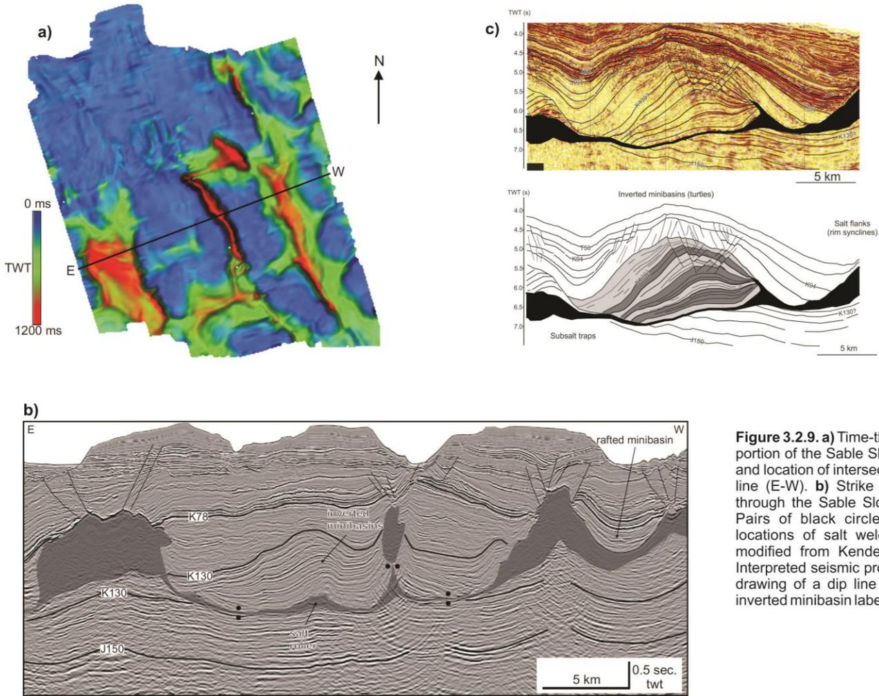
**Figure 3.2.9. a)** Time-thickness of a portion of the Sable Slope Canopy and location of intersecting seismic line (E-W). **b)** Strike seismic line through the Sable Slope Canopy. Pairs of black circles mark the locations of salt welds. (Images modified from Kendell, 2012) **c)** Interpreted seismic profile and line drawing of a dip line through the inverted minibasin labeled in (b).
