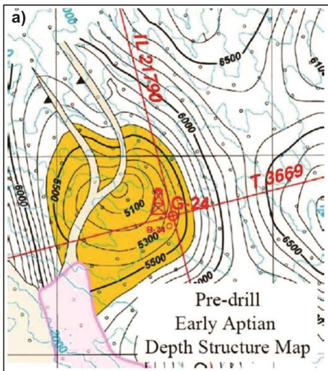
**Figure 3.1.2. a)** Pre-drill depth structure map of Annapolis G-24, as mapped by Marathon. Note that this map is of the early Aptian, the pay sands at this location were found in an older Hauterivian-Barremian interval. **b)** Seismic profile intersecting both the Annapolis and Crimson wells. (both images modified after Kidston et al., 2007)
