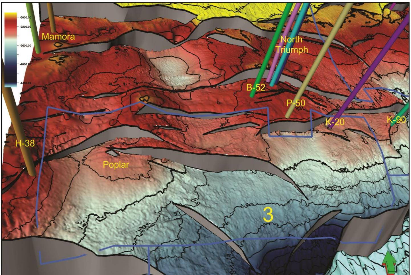
**Figure 2.4.2** 3-D perspective view of Hauterivian (K-130) time structure map on Parcel 3. Vertical exaggeration is 5X and contour interval is 100m. The Poplar lead is highlighted.
