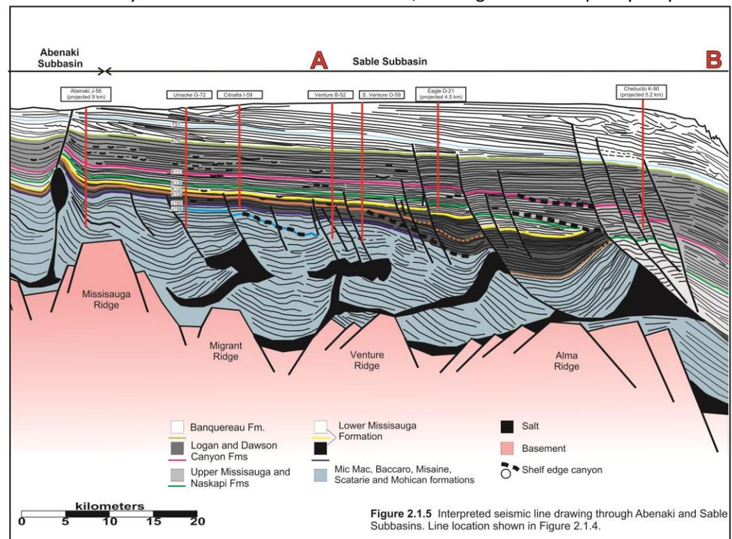
Figure 2.1.5 Interpreted seismic line drawing through Abenaki and Sable Subbasins. Line location shown in Figure 2.1.4.
