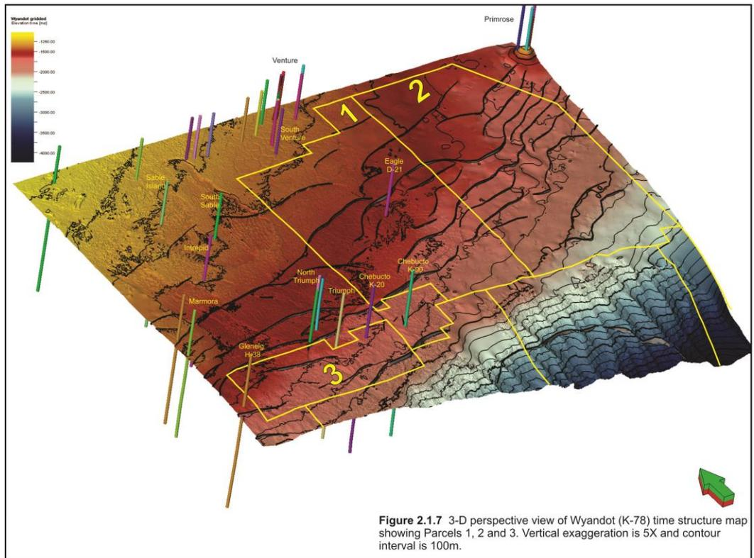
Figure 2.1.7 3-D perspective view of Wyandot (K-78) time structure map showing Parcels 1, 2 and 3. Vertical exaggeration is 5X and contour interval is 100m.
