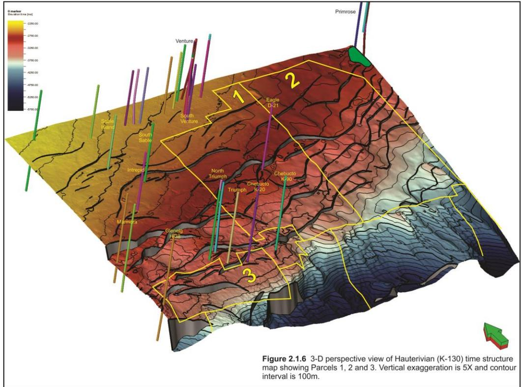
Figure 2.1.6 3-D perspective view of Hauterivian (K-130) time structure map showing Parcels 1, 2 and 3. Vertical exaggeration is 5X and contour interval is 100m.
