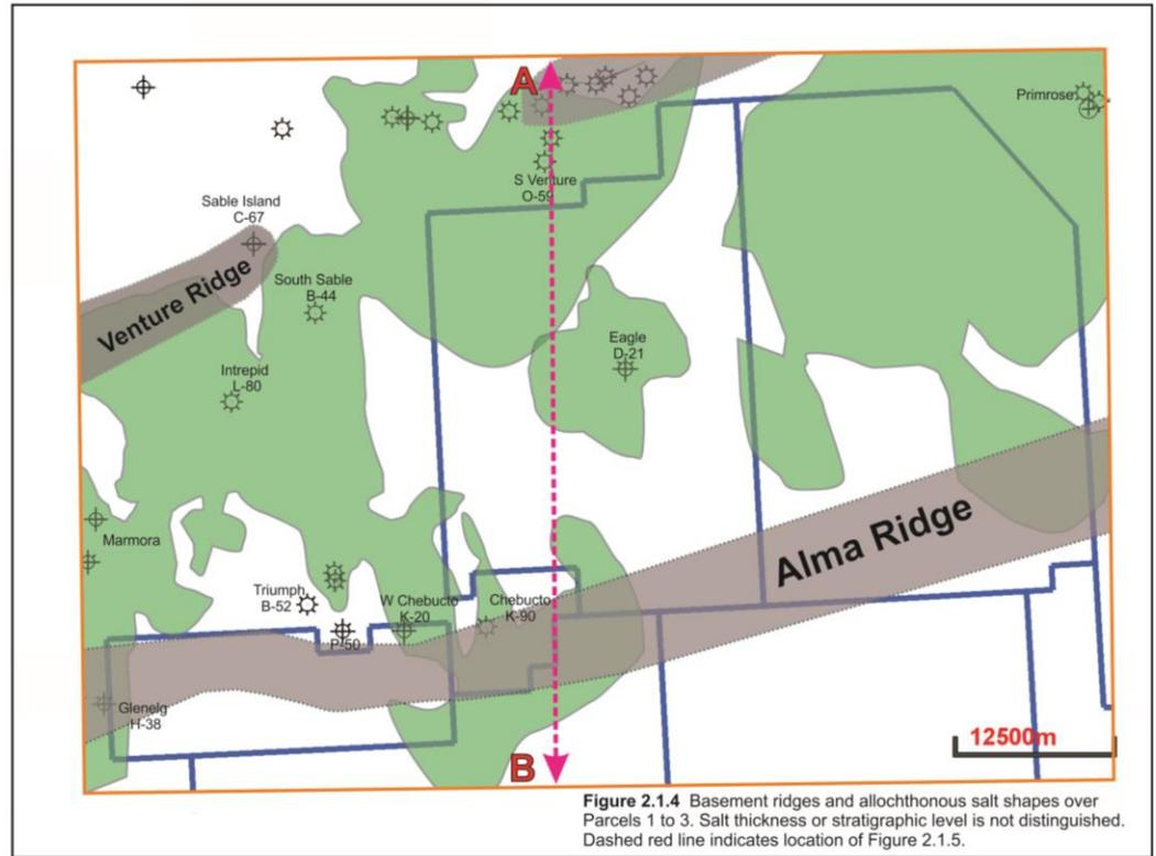
Figure 2.1.4 Basement ridges and allochthonous salt shapes over Parcels 1 to 3. Salt thickness or stratigraphic level is not distinguished. Dashed red line indicates location of Figure 2.1.5.
