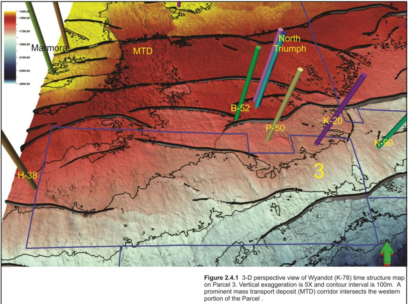
Figure 2.4.1 3-D perspective view of Wyandot (K-78) time structure map on Parcel 3. Vertical exaggeration is 5X and contour interval is 100m. A prominent mass transport deposit (MTD) corridor intersects the western portion of the Parcel .
