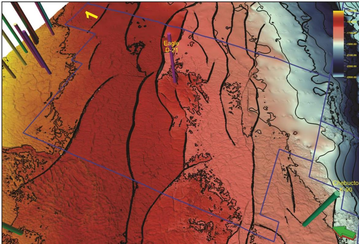
**Figure 2.2.2** 3-D perspective view of Wyandot (K-78) time structure map on Parcel 1. Vertical exaggeration is 5X and contour interval is 100m. Structural closure at Eagle is evident.
